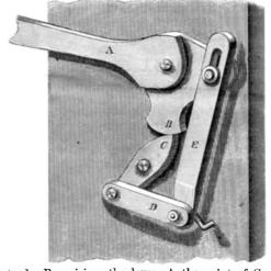
understood. By raising the lever, A, the point of C slides over the face of B and falls by the weight of the bar, E, be yond the radius, where the front of B takes it and reverses its motion; the bar, E, gradually rising until near the vertical center, when the reciprocating movement of A completes the turn.
