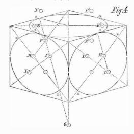
not shown, and the vertical ellipses from four centers H H' I I' (see Fig. 4), in which the  $15^{\circ}$  and  $37\frac{1}{2}^{\circ}$  angles are shown respectively by equal and unequal dots. The arcs marked \* are all of equal radius.
