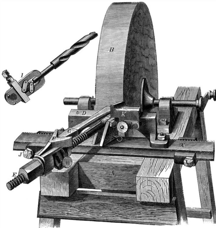
**STRAHAN'S DRILL REST FOR GRINDING.**
