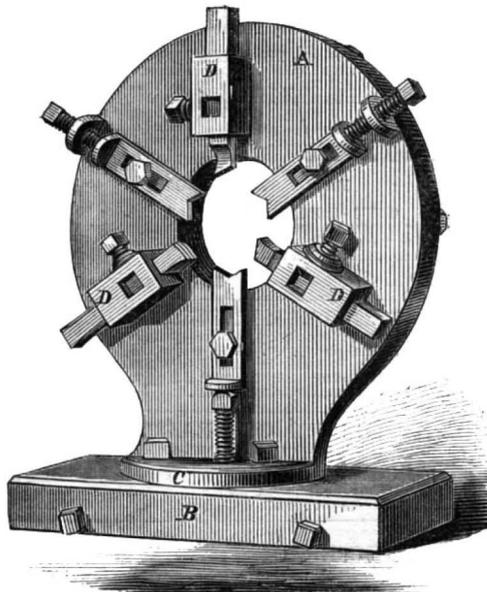
The object of the improvement is to avoid the trouble of removing bolts or studs from the lathe, after being turned, for the purpose of threading them in the screwing machine, which is a quicker way than that of chasing them on the lathe, but renders them liable to be threaded one sided.
