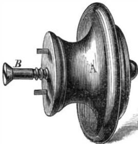
device, suffers some detraction from their liability to break off, or unscrew and become loose. To prevent this latter occurrence is the object of the improvement herewith illustrated.
