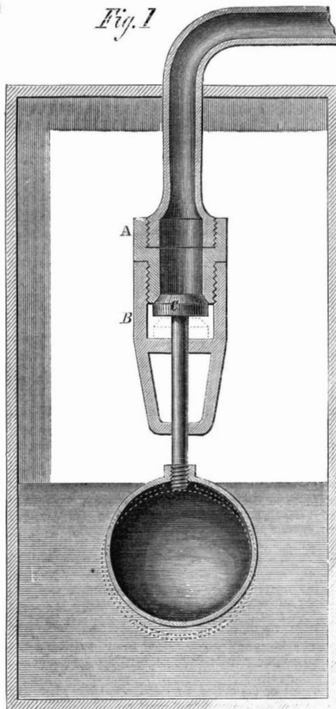
soon as separated from the seat, being practically nothing. Its action is also direct, and the float can always exert power enough to close the pipe.
