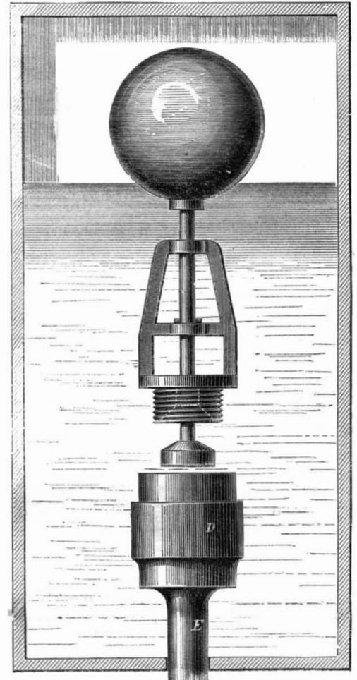
As the water falls, the float opens the valve and permits the further introduction of water through the pipe. So, as it rises, the valve is closed, the application of the power being direct.
