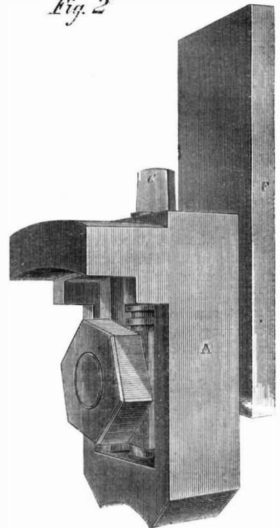
By the use of these adjustable and removable jaws the machinist can dispense with the cumbersome independent jaw chuck, which would be especially desirable for the proprietors of small shops. The overhang of the jaws enables the workman to chuck either from the inside or outside, and the graduating screw, with the adjustable jaws, will render the chucking of irregular shapes easy and convenient. The device is a good one.
