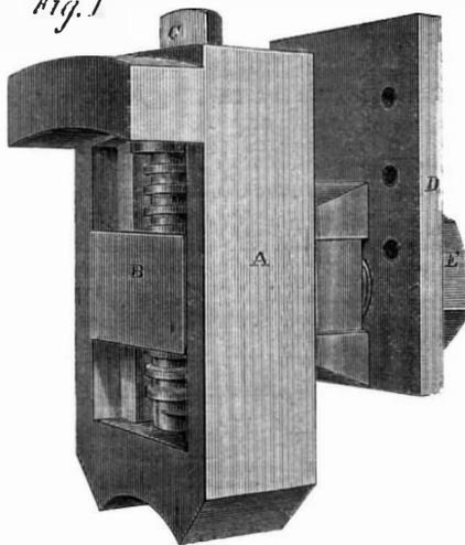
The jaw, A, is of cast iron, having a rabbeted slot in which slides the nut, B, through which the screw, C, works, thus raising or lowering the jaw from or toward the center. The shank of the nut, B, passes through the face plate and the back plate, D, and has a nut, E, on the end. Fig. 1 shows the form of jaw adapted for the face plate, having its radial slots cut entirely through. Holes are made in the back plate, which correspond to similar holes in the face
