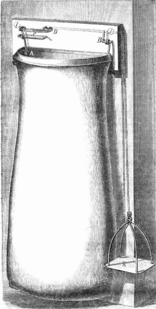
room or hung on nails to any upright—a wall, tree, etc. The corners of the wire are twisted, as at A, which gives a spring to the hoop, and while one end merely turns on the staple at B, the other has a sliding motion, also, on the long staple, C. To this end is attached a line which passes through the board at D, and along the back, as shown by the dotted lines, depending from the other end, and being furnished with a stirrup, E, for the foot.
