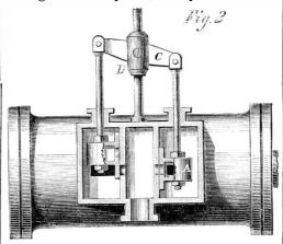
position, and the opposite end working through a egment with notches, so as to take a catch or spring to hold the valves when moved to the position for stopping, backing, or slowing the engine. A small model of a double engine is shown in the engraving. that was made simply for exhibition, and the reversing gear was arranged to accommodate the working of it. The cylinders stand only sixteen inches apart, from outside to outside, and are 2 inch bore and 4
