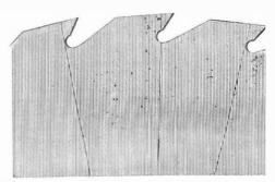
one inch and a quarter long, or deep, from the point. The under side of the tooth should range about eight inches from the center for hard wood, and ten inches for soft wood; or, if a large saw, twelve inches will not be too much.
