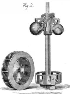
the end of a bell crank, D. The other end of the same connects with a coller on a cast-iron sleeve, E, fitting over the main shaft, and the governor levers also connect with it through the medium of a bolt, F. The sleeve, E, connects at the bottom of a regulator valve, G, Fig. 2.
