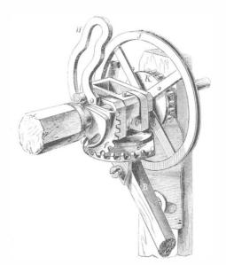
pinion, K, having an equal number of teeth, which causes it to revolve once on its own axis during each of its revolutions around the shaft of the reel. This imparts such motion to the crank on the end of the axle of pinion, I, as to bring this crank to the lower end of the slot in the arm, H, just as the rake has completed its passage across the platform, and then this crank, in its onward movement, carries the collar, C, and with it the rake, around the shaft of the reel.
