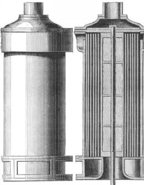
Fig. 16 is a condenser, adopted by Mr. Rowan, of Glasgow. It consists of a number of tubes, contained in a case, and surrounded with water, which is kept in motion by a fan or agitator. To this agitator is due the superiority of this over other condensers.
