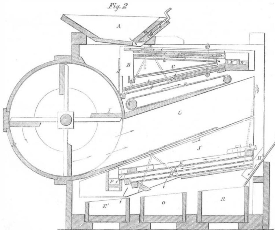
upper sieve, *e*, through sieve *f*, on to the imperforated plate, *v*, of sieve *g*, thence it slides on to the wire screen, *h*, which separates the grass seed from it, the grass seed passing through the meshes of the screen on to the inclined bottom, *c'*, thence into the trough, *q*, whereby it is conducted out one side of the ma-
