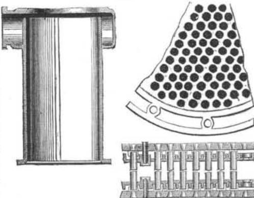
In early examples it was proposed also to mix air with the water, but this is not adopted in practice. The exhaust steam from the engine enters at the top. The water passes through a screen of wire gauze, to intercept all extraneous matter. The value of this screen was exemplified by the fact that, although placed, in early condensers, at an angle to give it more
