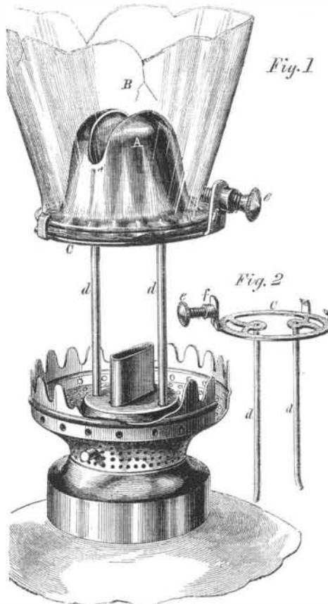
considerable elasticity, enabling the screw to yield to any expansion of the glass, and thus prevent the chimney from cracking. This is a very important matter, as a great many chimneys are broken, either
