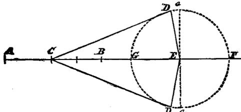
Suppose the line  $x$  (C D) be applied to A G, or we start with the crank at G. Now carry it forward on the line A F, till D coincides with E, and the line  $x$  with C E. It is evident that C will be at the middle point of A B. Now elevate the point D along the perpendicular E e, to the point e; it is equally evident that the other extremity of the line  $x$  will approach the center, E, equal to the distance from E to the foot of a perpendicular let fall from the point D on the line A E.
