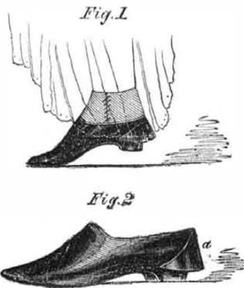
thrown up by the foot strikes against the underside of the shield; and thus the outer side, which comes in contact with the clothing, is kept perfectly dry.
