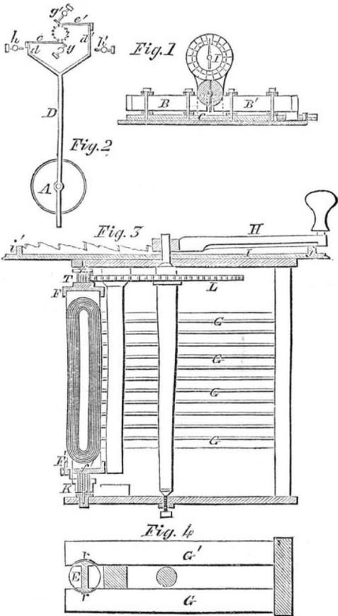
The hooks, e e', are furnished with projections extending beyond the wheel, and bent down, which strike against screws, g g', whenever the motion of the arm, by coming in contact with the set-screws, h h', has arrived on its extreme point. By these means, the progress of the wheel beyond the required distance is prevented.
