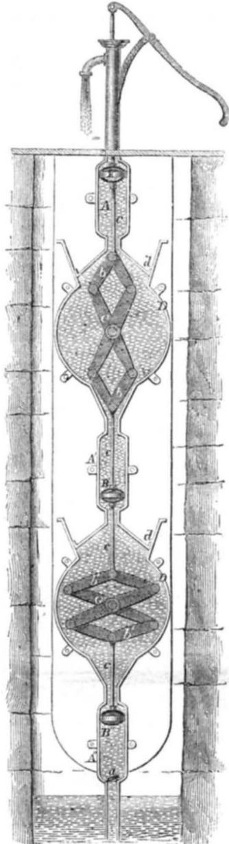
water from the well is drawn up. When *B* is depressed, it passes through the water in *A* by its clack valve being opened, and compressing the rods, *b C*, elevates the piston, *B'*, thus bringing up more water, and at the same time the opening of the cross-rods and links, *b'* and *C'*, depresses the piston, *B''*, and the weight of water closes *a*.
