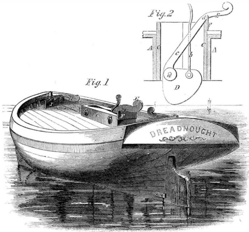
enabled to sail closer on a wind, and hence be much more under control and enabled to be kept from a lee shore. The oblique direction of D must be changed every time the vessel is in stays. As an auxiliary to D, the cut-water, G, is made to project from the vessel and to be movable like a rudder, that it may be set to windward like the center-board in
