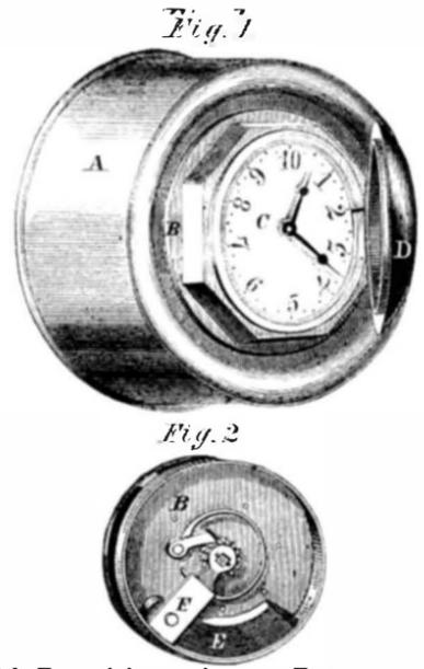
dial; E remaining stationary. To the center of the end of F, where it is pivoted to the gearing, a small ratchet wheel is attached, and this by a pawl and spring that tends always to keep the pawl in the teeth, prevents the weight from registering when the vehicle is backed. This little piece of mechanism is so simple that it can be understood at a glance, and there is no fear of its getting out of order, but it will run from year's end to year's end with perfection.
