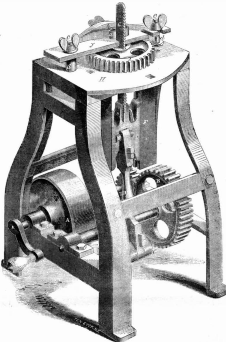
secured to it by clamps passing through the table itself, as well as by a permanent clamp, J, that is held down on the wheel by the screws, d, and nuts, c. The saw, G, works up and down in a slot in J, and it is pressed against the inner periphery, or provided with the requisite feed by a spring, a, that can be
