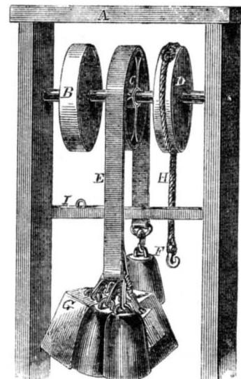
Leather belt on iron pulley slipped at 48 lbs.
