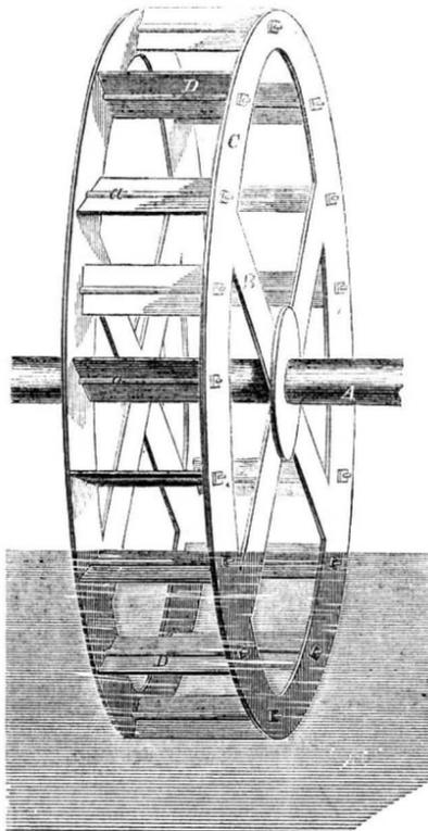
The shaft is seen at A, and on this shaft is supported a wheel, C, by arms, B. The two sides of this wheel are braced together by cross bars, *a*. The buckets or floats are formed of boiler iron or wood, having a circular channel running through their centers horizontally, through which is passed the cross bar or tie, *a*; and the buckets being perfectly balanced on *a*, can rotate freely on them.
