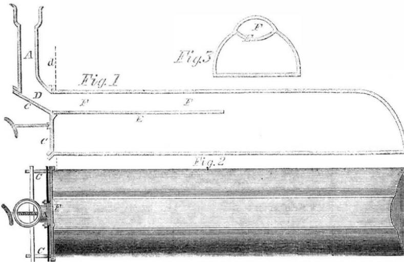
head and screw. A flange, E, runs under F for about half the length of the retort, and forms a kind of pipe, to relieve the back of the retort, and as the gases from the front have also to pass through it, they are kept much longer in contact with the heated surface.
