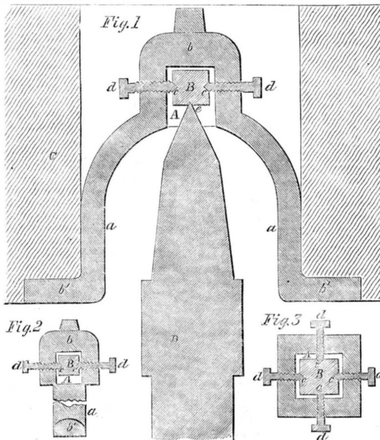
The ordinary or common bail used as a bearing for millstones is permanently secured in the eye of the stone, and when a new center hole is required, the balance iron has to be detached from the stone at considerable expense and trouble, and then replaced in the stone, and balanced by adding weights on the light side, an operation that is extremely troublesome. By the improvement which we are about to describe this inconveni-
