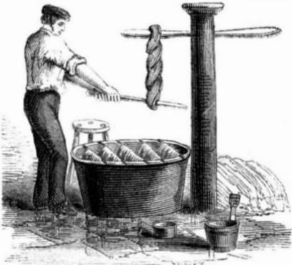
the processes. The accompanying figures represent two different operations. Fig. 1 illustrates the manipulation of yarn or skein dyeing; Fig. 2, that of dyeing cotton or woolen cloth in the piece. The operative, in Fig. 1, should stand square before the arm of the post, but this position would have covered the tub.
