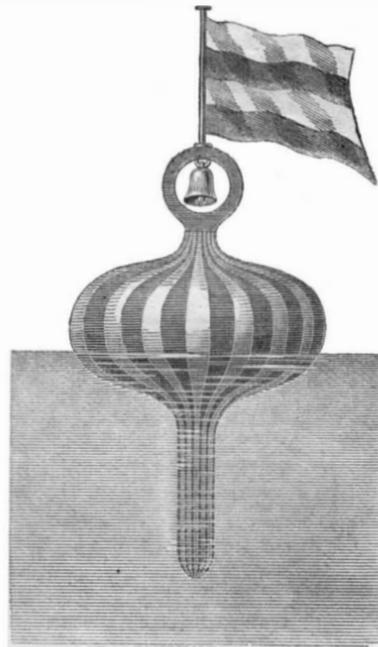
capable of resisting any ordinary pressure. Within this hollow space or chamber it is proposed to insert a slip of paper or card, or any other document, and even property, if made large enough, when all hope of safety and rescue shall fail, and at the final sinking or breaking up of the ship, the buoy would float off, with the probability of being picked up at some time.
