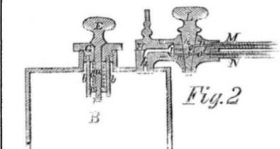
close to its seat; but when the pressure becomes greater than the power of the spring, the valve is elevated, and the vapor escapes. The pressure can be regulated by the compression of the spring, but it is so arranged that it cannot be compressed beyond a certain point.
