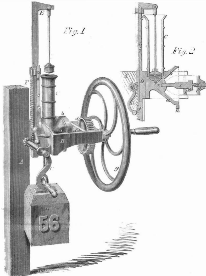
Although paint can be ground very finely and well with a muller and stone, yet the operation is very tedious and slow, and it has been found advisable in this, as in every other branch of manufacture, to introduce machinery. Our engravings illustrate a mill for grinding paint with expedition and evenness.
