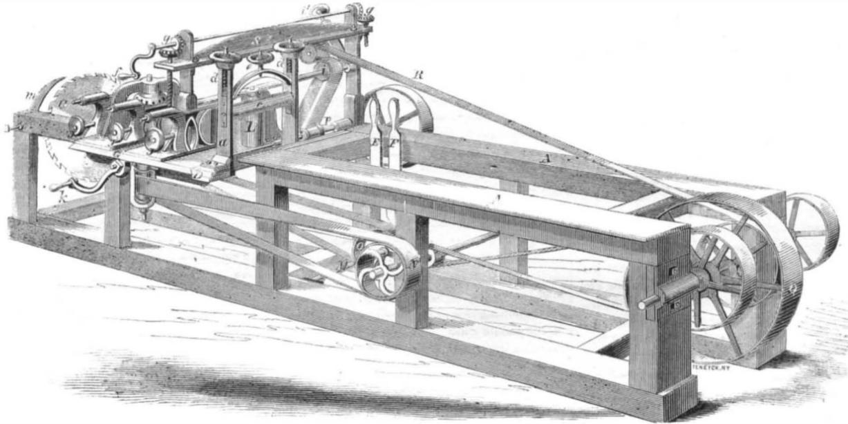
This machine is intended for re-sawing boards of any thickness into "siding," and planing, jointing and sawing the "siding" or lapboards at one operation.
