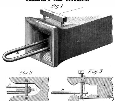
We have often had occasion to point out | box, A, having its mouth flared as usual, and the advantages which would be obtained by the use of some improved coupling that would prevent the necessity of persons passing between the cars when liable to move, to couple them, and that would allow of the cars being easily detached from the platform, in case of accident. We now reiterate the enumeration of these desirable ends, and proceed to describe the coupling which is the subject of our engravings.
