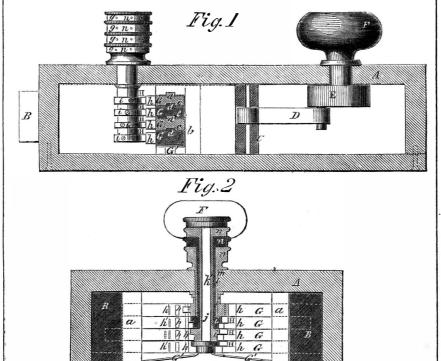
This invention consists in the use of a series; one, and from them and the following descripof slides provided with teeth or racks, and arranged with a bifurcated bolt into the parts of which the ends of the slides work or pass, and a series of bits attached to separate arbors placed one within the other, and operated by means of keys or knobs.
