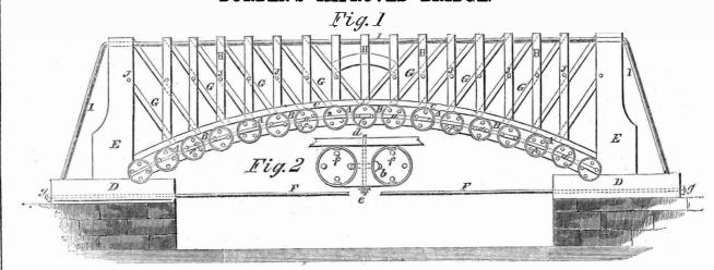
bers, and at their upper ends to the upper part of the posts, H H, and also notched and bolted to such of the posts as they pass. F are wrought iron tension rods passing through all the posts H and E, and down to the sills, D, to which they are secured by nuts or keys. J are the roadway-bearers which may be of wood or iron, having bearings at their ends in the posts.
