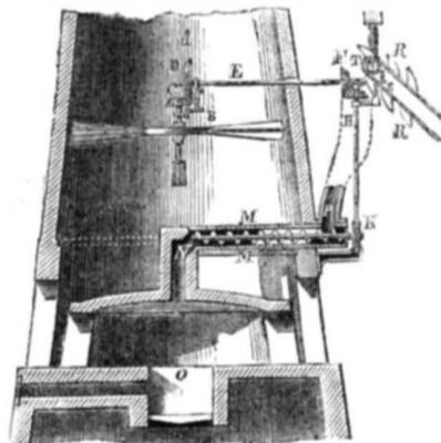
itself. A is the cone of the glass stack or house; it is furnished with a screw fan-wheel, B, set in the wall, and revolving horizontally in the stack. The bevel gear, C D, operated by the fan, gives motion to the shaft, E, on which are gears, F G, that give motion to the vertical shaft, H, the lower end of which has a worm wheel on it that meshes into another,
