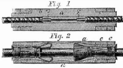
screwed on to each end of the tube to press and secure the ends of the cable. The junction is made between the sections of the cables by bringing them together in the tube when nuts are slipped over the ends of section cables, thus allowing the jointed parts, *b*, of the tube to be opened so as to permit plastic gutta percha to be filled around the cable. The jointed parts, *b*, are then shut down, the nuts pushed off the cables upon the tubes, then screwed up, and the junction is complete.
