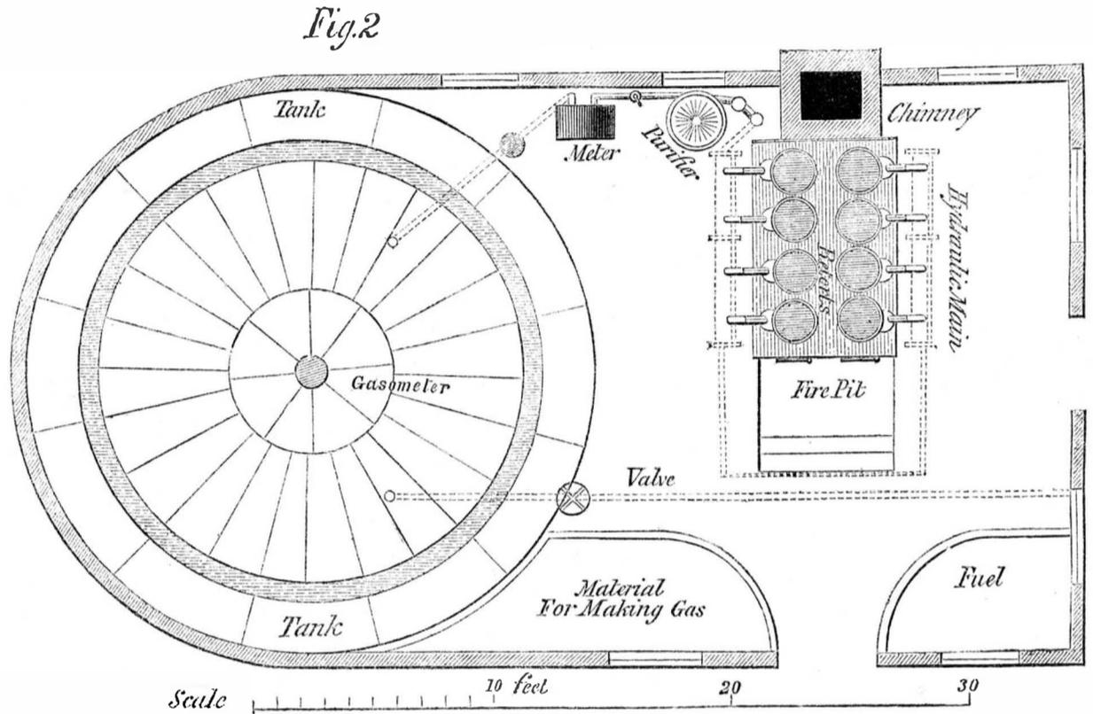
fier, and gas-holder, from which it is distributed in the usual way. As long as any volatile matters remain in the charger, an oscillating or dancing motion is kept up, by which it will be understood that a more thorough decomposition of the vapors is secured, since no vapor can possibly escape without passing between two red-hot surfaces;
