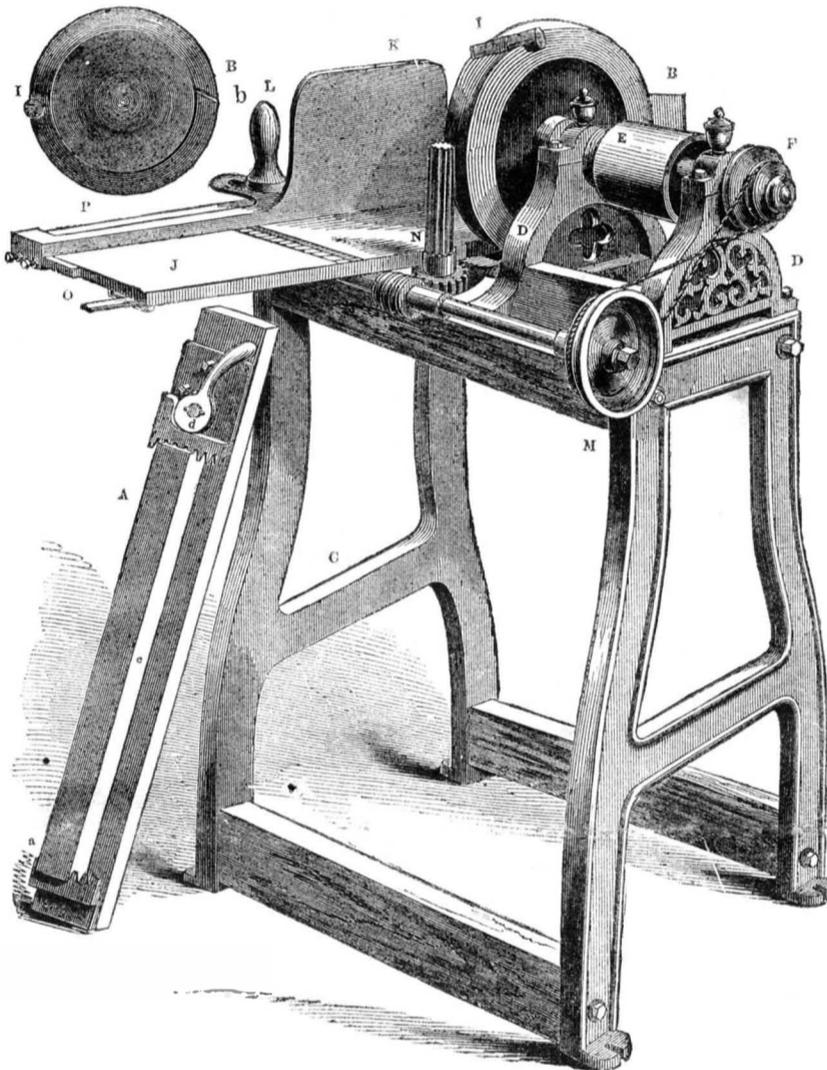
These planers dress lumber of all descriptions to any desired thickness, bevel or taper, at the rate of about thirty feet per minute, and also take the "wind" out, leaving the surface smooth, and the corners perfect. They are remarkably simple, and not liable to get out of repair.
