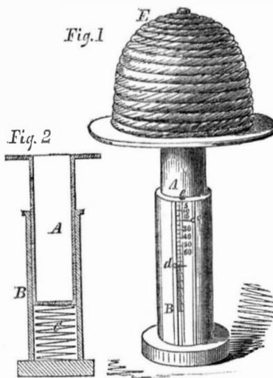
finger, d, is attached to the base of the pillar, and the slit in which it works is quite open; so that as A presses down the spiral spring, the finger, d, marks the gross weight of the hive, hive-board, sufers, bees and honey. At e a thumb screw passes through the rim of
