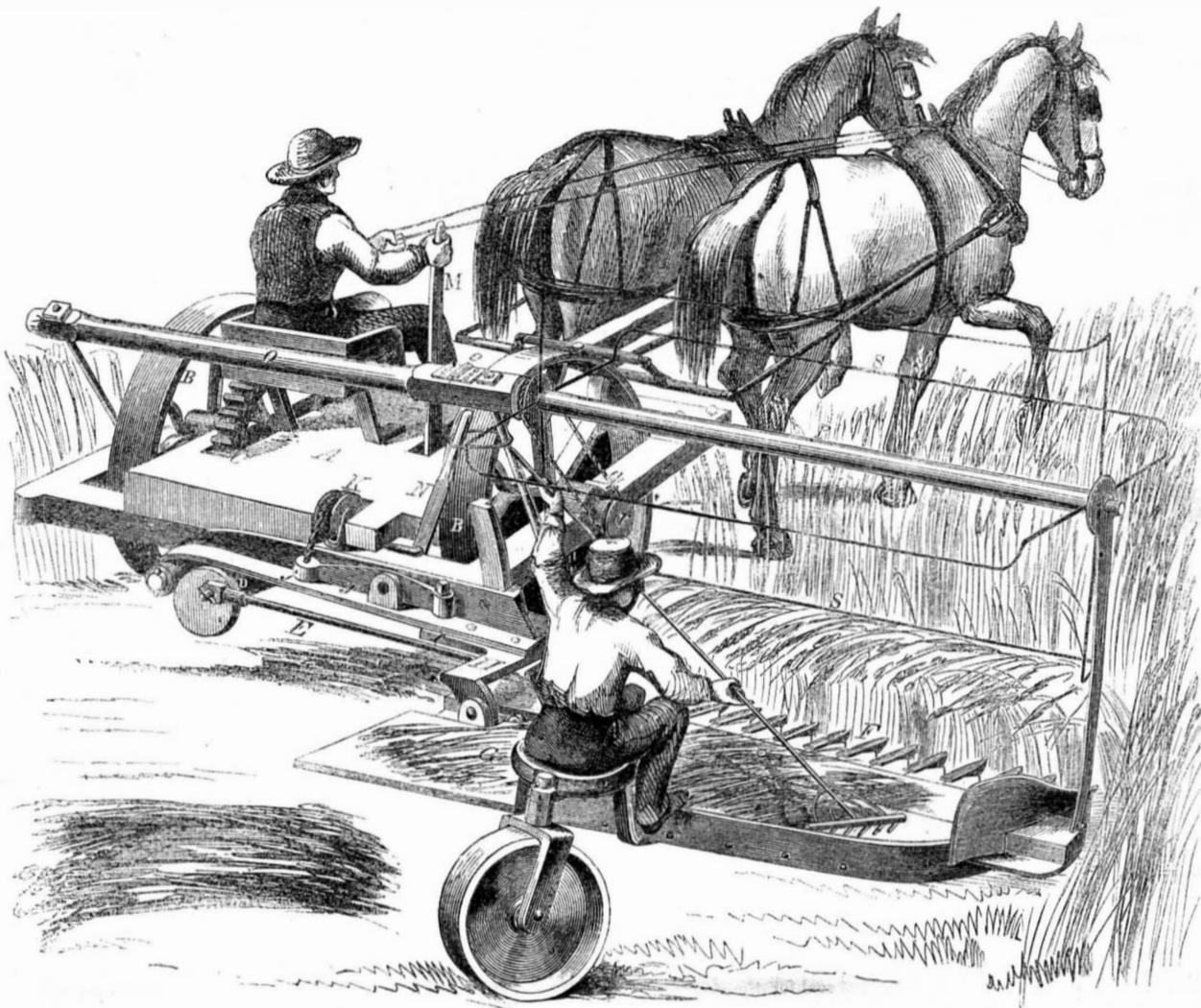
platform being well and strongly hinged to the casting, H, which is firmly secured to A. G has a tongue, or piece of iron, I, projecting from it, on which the screw in the end of the lever, J, can exert pressure, by means of the cord, k, passing over the pulley, K, and worked by the lever, M, so that the platform, G, and cutters, F, can be raised or depressed
