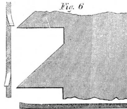
understood among sawyers as to require no description from us. In this case, after the tooth is worn off so as to be thinner at the point, it may be spread out to its original thickness with the crotch punch.
