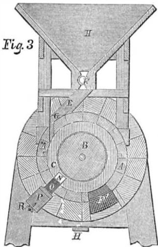
adjustable strip let into the lower side of the case A, and on which are fixed plates O, so that when P is raised by the thumb screws, R, to its highest position, the plates O nearly or
