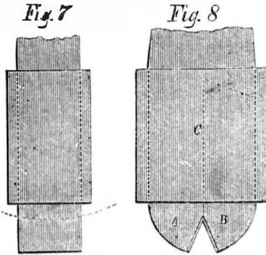
bound together with the iron band, C. It is used to widen the points of saw teeth when they have become worn and blunted on the corners, and may be used without the necessity of filing the saw afterwards.
