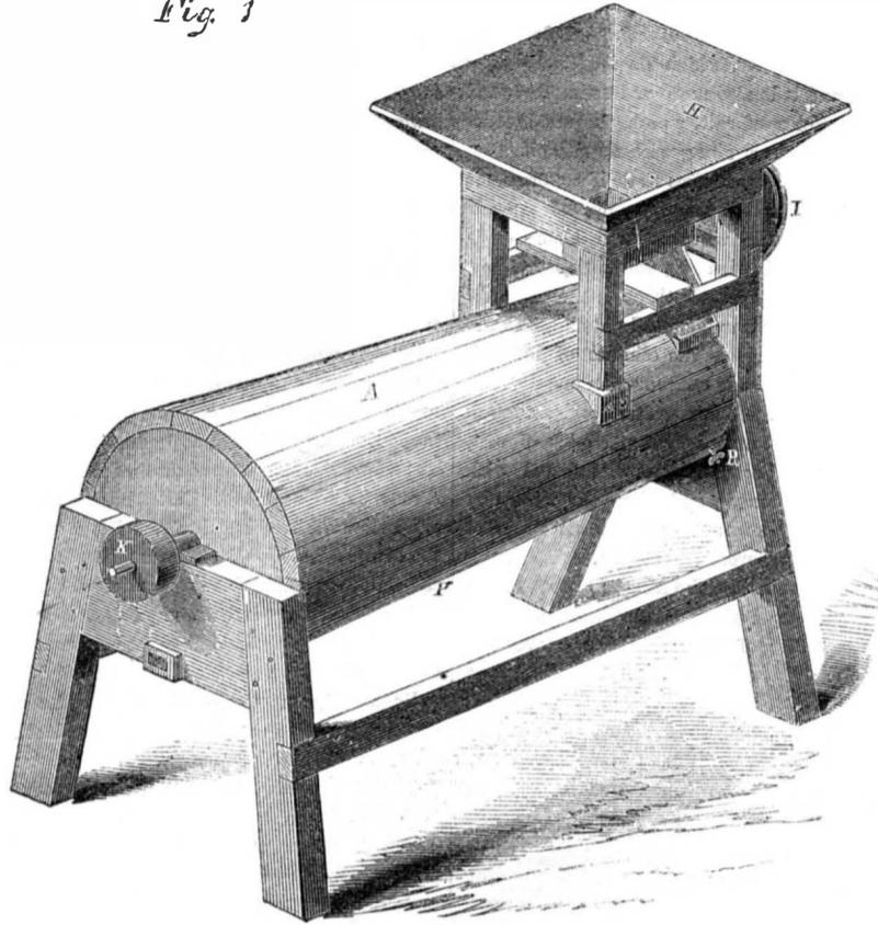
parts. A is the case or concave which may be of wood in either one or two thicknesses lined with metal. B is the drum or conical "cylinder," and C the rings fixed in A. N. Fig. 3 shows the opening in C through which the grain finds its way at a proper rate, regulated by means explained below. D represents the pegs or beaters which are only shown
