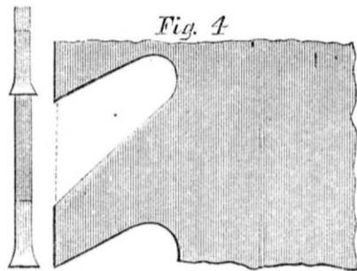
must be set and sharpened in the same manner as circulars. The pitch of the teeth is 60 degrees.
