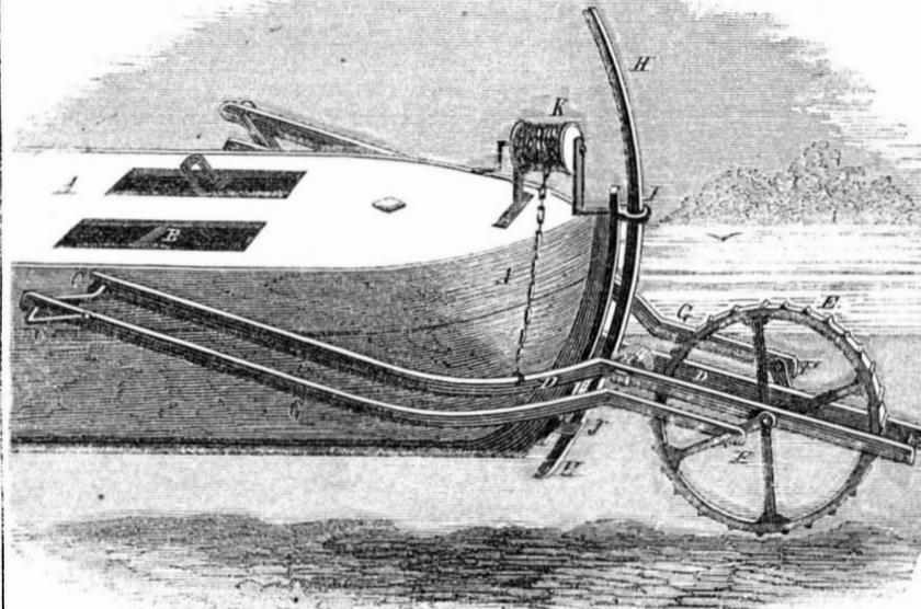
onward, somewhat in a manner analogous to the motion of a locomotive. The frame allows the wheel to rise and fall to accommodate itself to the inequalities of the bottom.
