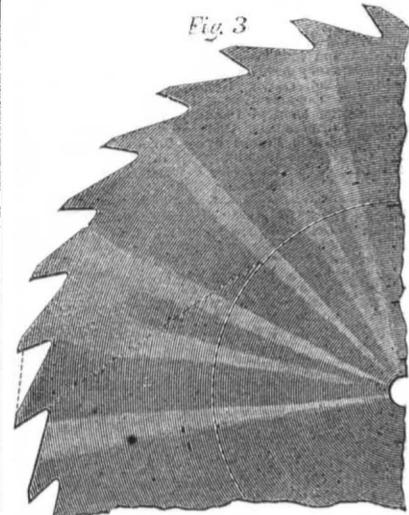
be filed up sharp, finishing with a fine, single-cut file. The cutting edge of each tooth should be parallel with the center of the mandrel, and the front and back of the teeth kept on the lines as described, and shown in Fig. 3.
