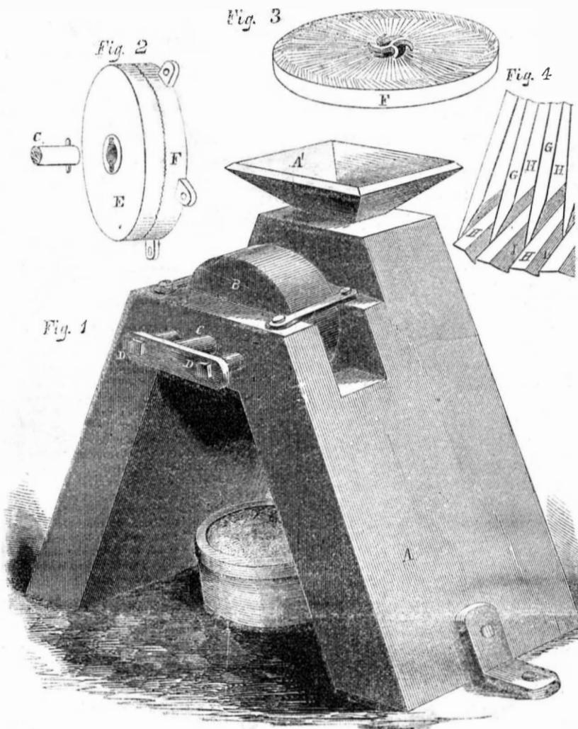
The accompanying engravings represent a very cheap and simple metallic mill to be operated by hand or power, and mainly intended for coarsely grinding grain for farm use.
