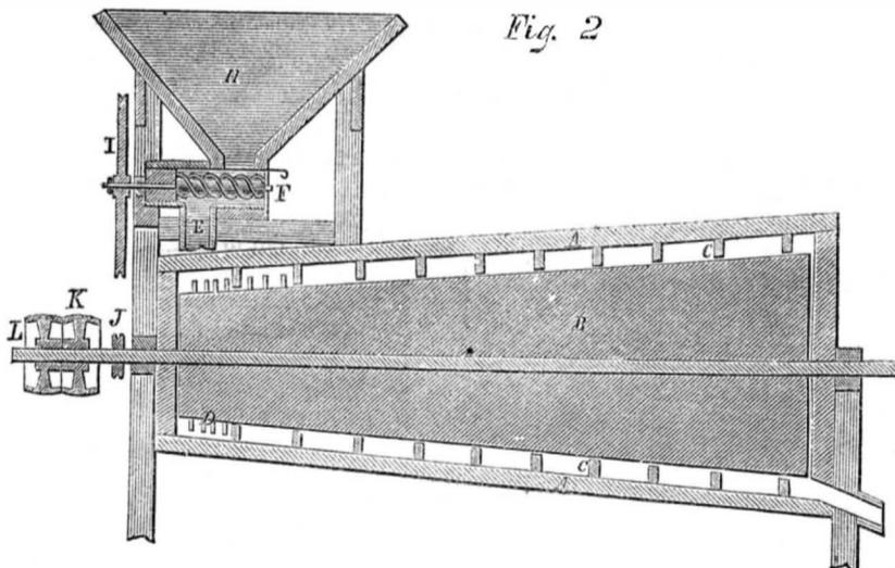
and loose pulleys on the shaft of B, by which it is driven. F' is a screen through which any dust may be discharged. P represents an
