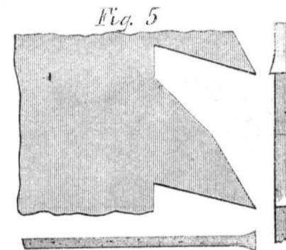
edge, the teeth are filed sharp at the points, like a cross-cut saw, alternately highest on the outside, and then upset with the punch.
