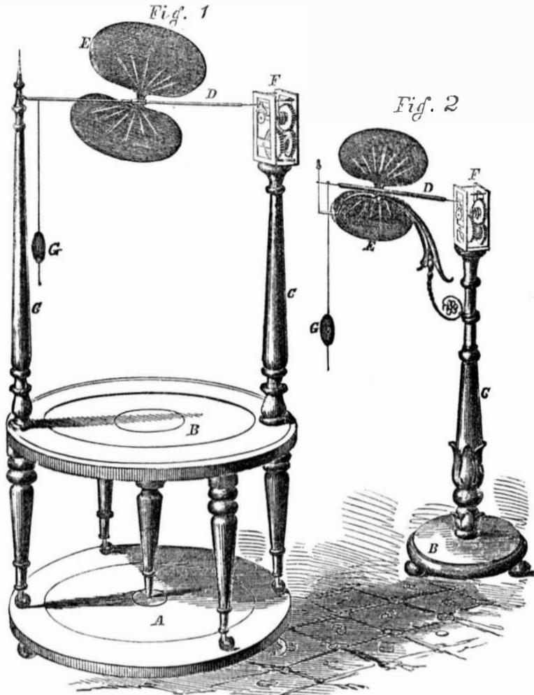
two broad thin wings of paper or other suitable material, F strong clock-work, and G a pendulum fixed on D. The effect of the clock-work is to give an active reciprocating motion to D and consequently to both E E and G. The motion agitates the air and produces the effect desired. By turning the
