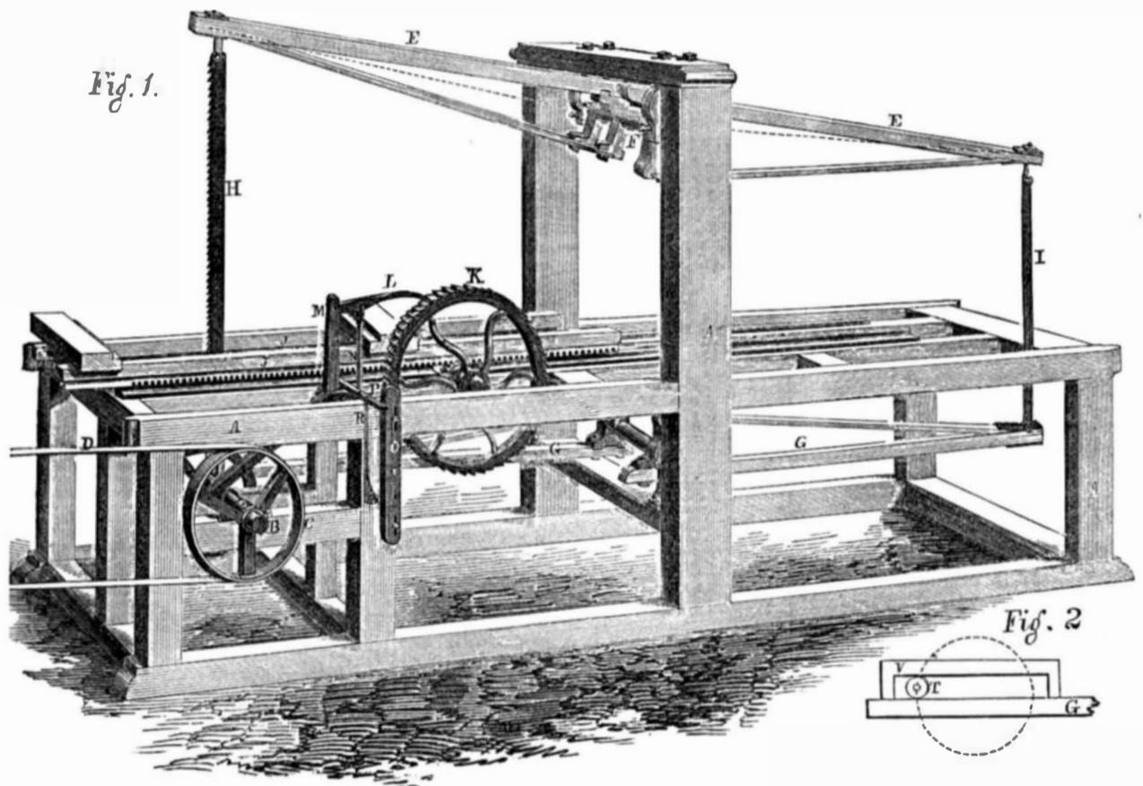
The mill represented in the accompanying engraving is the invention of Carlyle Whipple, of Lewiston, Me., and was patented on the 13th of January last. In it, the saw is stretched between two reciprocating levers, each resembling the walking beam of a steam-boat, the means by which the motion is communicated being represented separately in Fig. 2.
