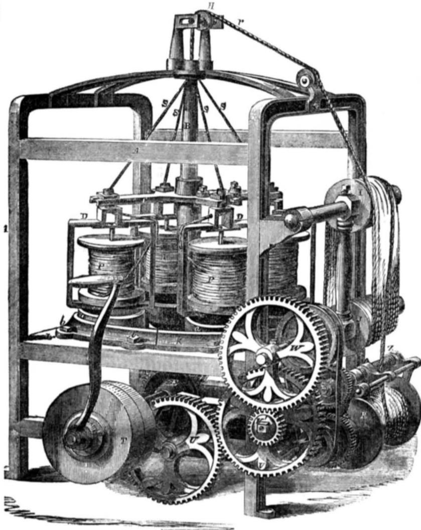
The accompanying figure is a perspective view of the improved rope-making machine, for which a patent was issued to Milton Wallwork on the 7th of April last. The improvement relates to the "sun and plane" rope machine, and consists in the means of controlling the speed of the strand flyers, for enabling the twist of the strands to be varied with facility. The figure represents the application of the machine to laying rope in a very small space, obviating the use of long rope walks.
