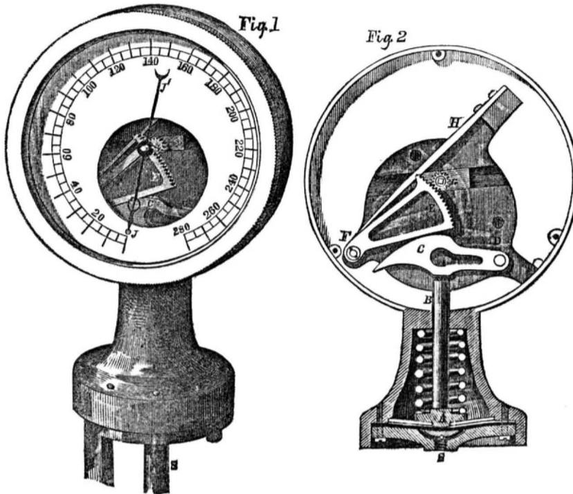
means indicates exactly the pressure. H is a slender spring, which acts on E with sufficient intensity to overcome the slight friction and insure its falling back, whenever the pressure of the steam is lowered and B is depressed by the action of the stout coiled spring.
