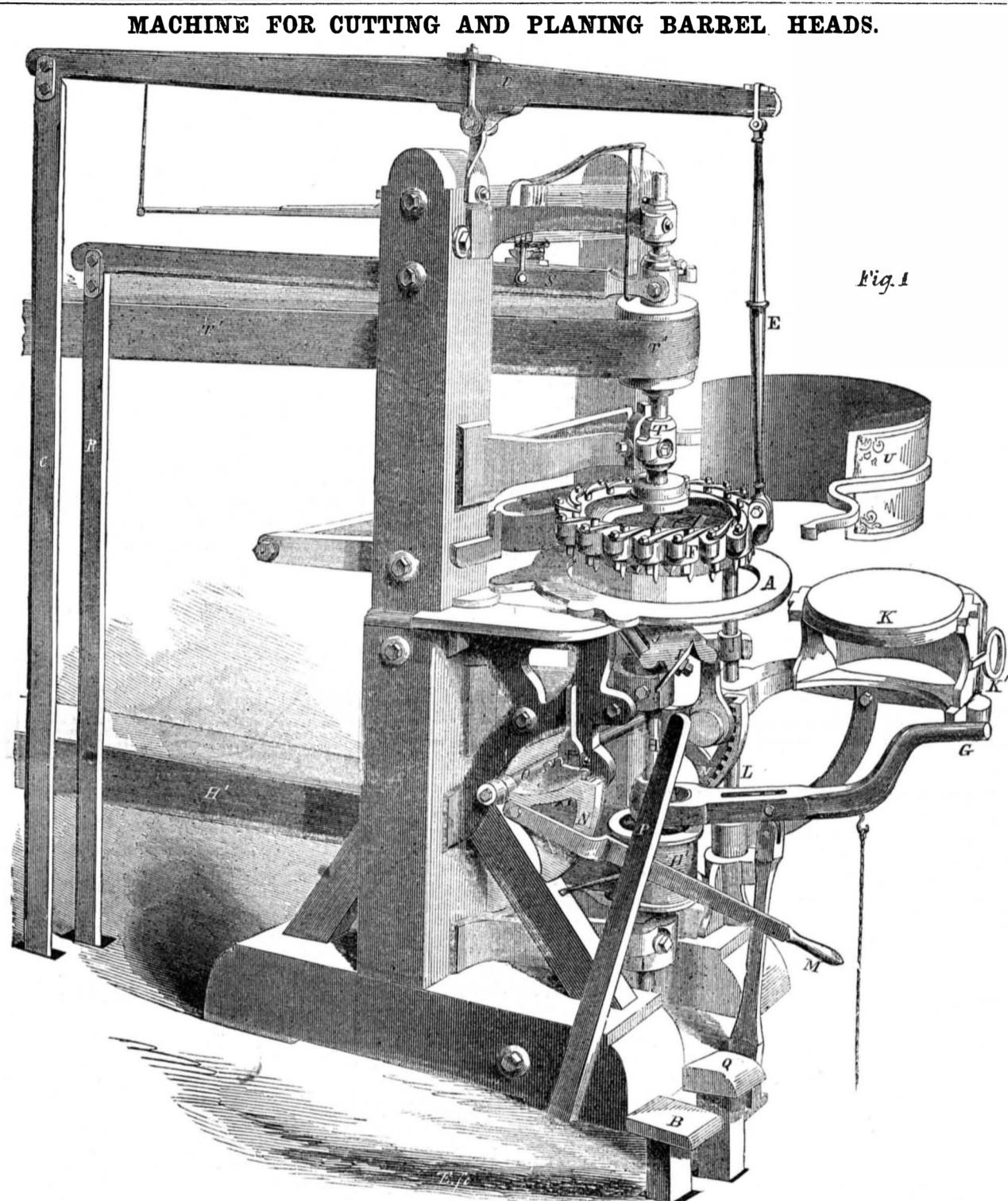
M is raised, it locks into a notch in rod P, and continues to hold bed K against the bottom of the boards.
