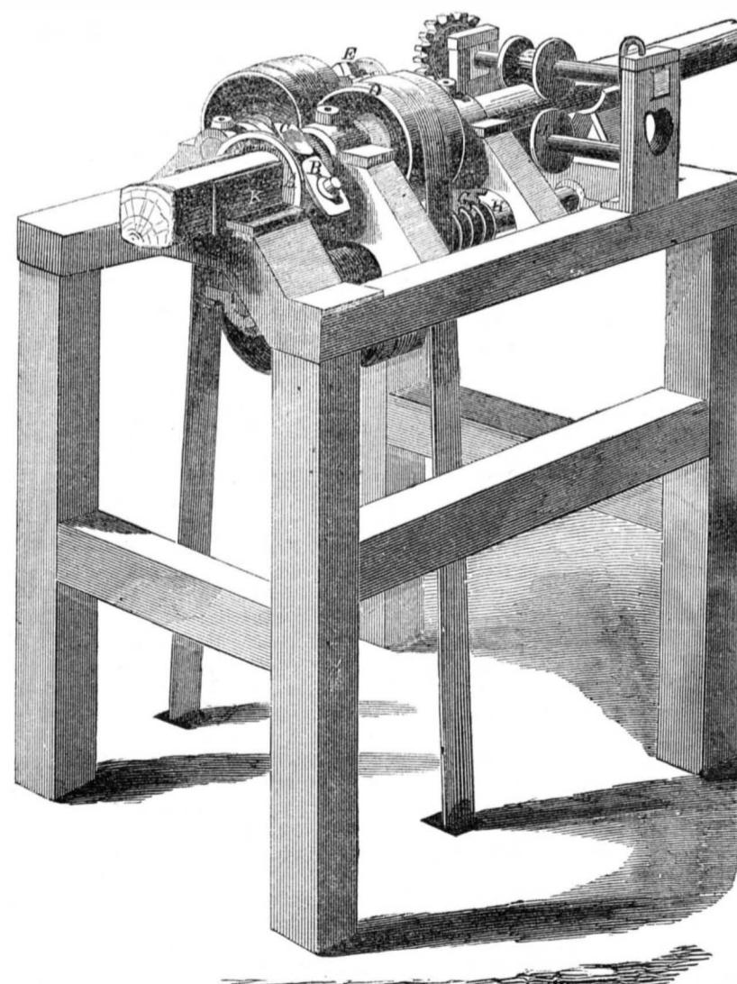
New Bedstead Rail Machine. Our engraving illustrates a machine for turning Bedstead Rails, now on exhibition at the American Institute Fair, Crystal Palace N. Y. It is the invention of T. R. Bailey of Lockport, N. Y. Patented July 25th, 1854.
