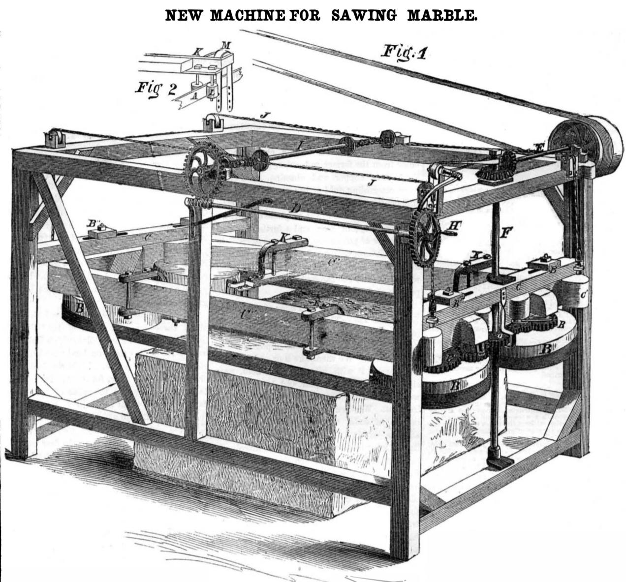
told that this machine cuts about three times faster than the common marble sawing apparatuses. The endless saws may be driven at a high speed, their motion is always steady,
