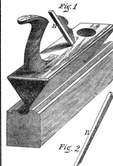
The plane stock, A, it will be seen, is made of triangular shape, and the cutting tool, B, which is quite narrow, projects at the apex of the angle. The plane is moved like the ordinary tool.
