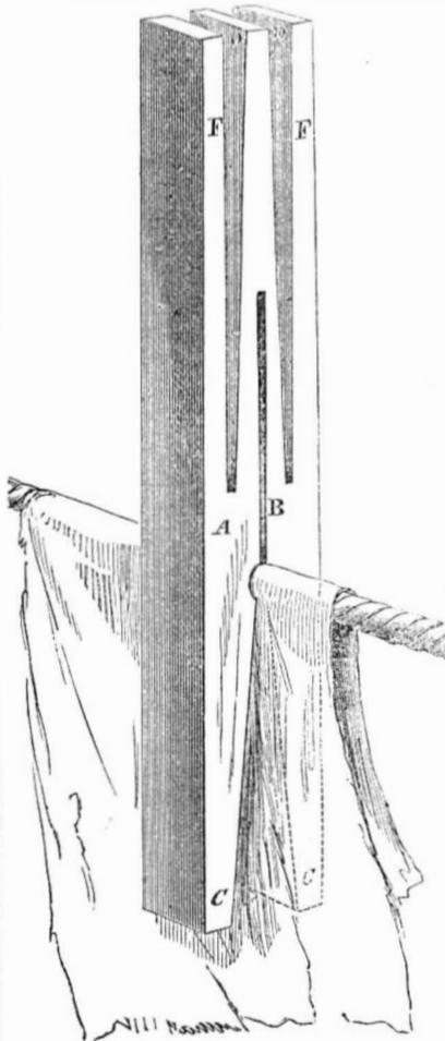
In securing clothes to the line, the lower jaws are extended to their fullest extent, by pressing the prongs, F, together, and the jaws, C, opened, and placed over the clothes, the
