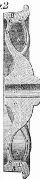
C, in one flange, come opposite the solid portions in the other one, so that any fracture would have either to pass through the wide part of one of the flanges, or to run obliquely across the tread of the wheel.
