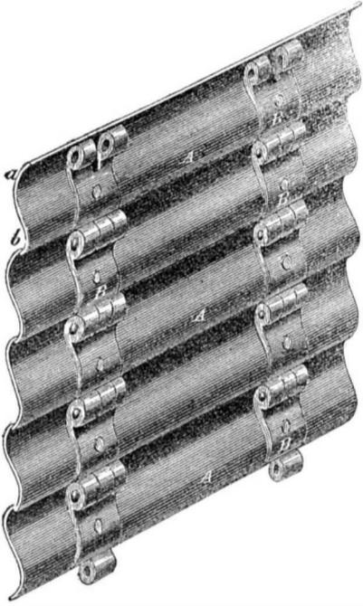
A represents the slats of the shutter connected by hinges, B, which are secured to the backs of the slats.
