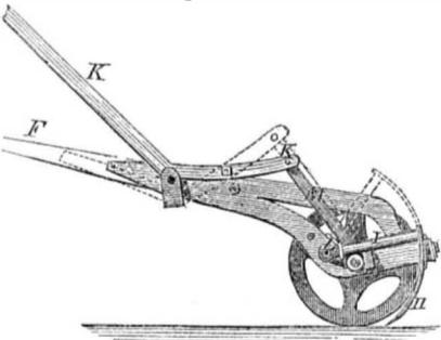
H are the rake teeth, made in curved form and attached to arms, I, which are pivoted at L. M is a connection rod which unites arms, I, with lever, K. By pressing down lever, K, the rake arms, I, with the rake will be elevated, and *vice versa*. A pin may be used at any convenient point to fasten K down, and keep the rake elevated, when desired.
