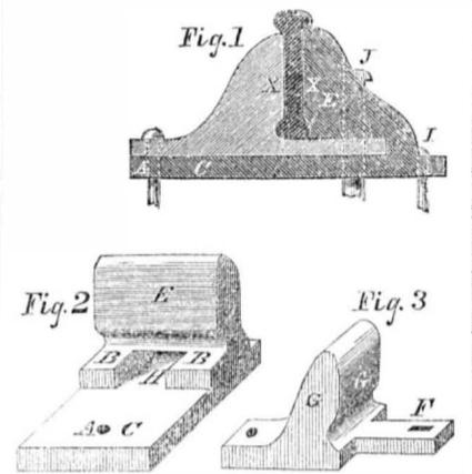
In the illustrations, fig. 1 shows an elevation of the chair when fixed; the dotted lines show the slide tongue and cotter. Fig. 2 shows a perspective view of the chair with slide withdrawn so as to admit of the rail being taken up or placed down; and fig. 3 shows a view of the slide and tongue part of the chair.
