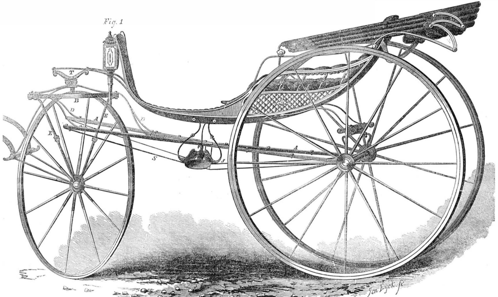
to getting in and out, and as the motion of this third wheel is not limited, the vehicle can be turned as short round as a vehicle on two wheels, and without the least cramping or straining of the body, or any part therewith connected.
