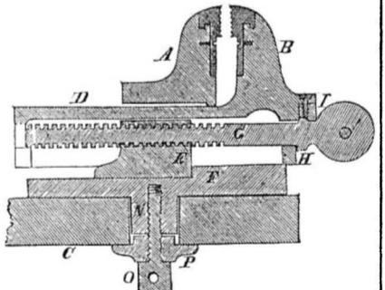
it passes through a groove or slot in the fixed jaw, A, and is made hollow, and in its motion slides over the screw box, E, fixed in the bed plate, F, the said bed plate being made in one piece with the fixed jaw, A; G is the screw by which the motion of the jaw, B, is produced. The screw, G, is situated nearly in the axis of
