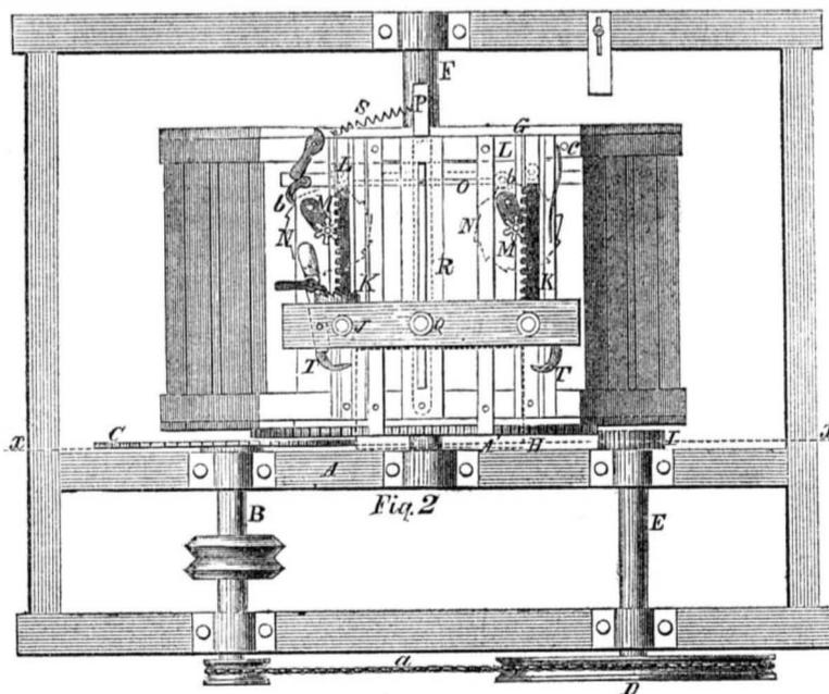
attached to it, said pawls catching into the ratchets, N. P is a lever, one end of which is pivoted to the under side of the face of the wheel. The bar, O, is attached to this lever, and the outer end of the lever, P, projects some distance beyond the side of the wheel, G. Through the center of the carriage, J, there passes a bolt, Q, the inner end of this bolt works in a slotted plate, R, attached to the
