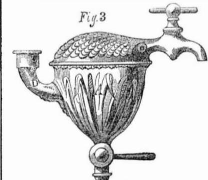
of dirt on one side of the filtering material. The present improvement overcomes that difficulty, in a great degree. Fig. 3 shows the external appearance, which may be rendered highly ornamental. The invention is applicable to large cistern reservoirs, and the purification of rain water. The form here shown is chiefly intended for city use. Patented July 1, 1856. Apply to the inventor, 835 Broadway, N. Y., for further information.
