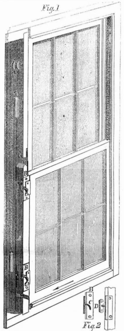
Both window sashes are constructed and hung with weights in the usual manner. One portion of the stile, A, is made movable; its ends are furnished with metallic plates, B B', in which curved slots, C, are cut. Button headed pins, D, attached to the frame, fit the slots, C. See fig. 2.
