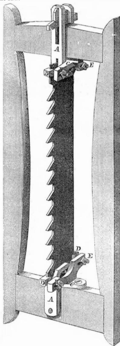
Each end of the saw is held by two stops one in front and one behind. By turning the nuts, E, which secure the stops to the saw, the stops will be changed in their position and the saw adjusted accordingly. The common method of holding saws is to drive wooden wedges between the saw and the stirrup.
