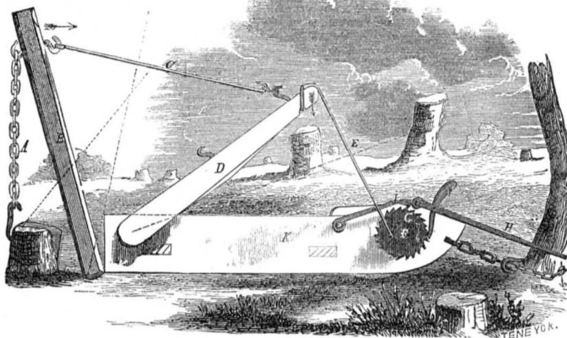
and prevents the ratchet wheel from turning back. By the winding of strap E on shaft F, the lever, D, is brought down, strut, B, raised to a perpendicular position, and the stump pulled. Most of the parts are attached to the sled, K, on which they are conveniently transported from place to place.
