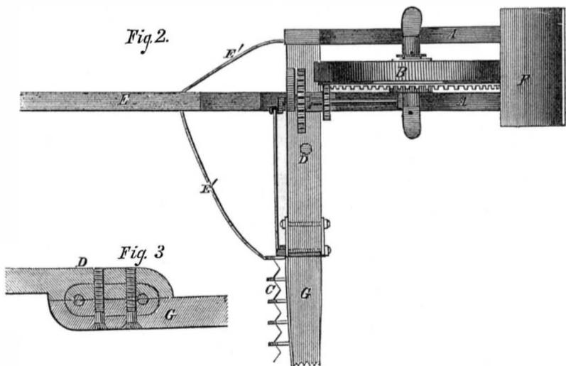
chine is rendered very compact. The method of constructing the frame and attaching the tongue is at once simple, strong, and economical in construction. The joint between bars D and G is also cheap, but very strong. This invention possesses several valuable features, and will, no doubt, find favor among agriculturists.
