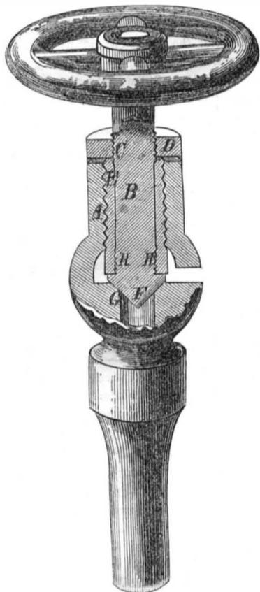
Referring to the above engraving, the improvement consists in having an outer shell, E, shipped over the spindle, B, and fastened as shown, at the screw threads, H H, and further secured by a flat nut, D, screwed hard against the end of shell E, at the thread, C. By turning back the hand wheel, the valve, F, is opened, or run back from the seat, G, allowing the steam or water to pass out through the opening below; the part, I, should be six-sided.
