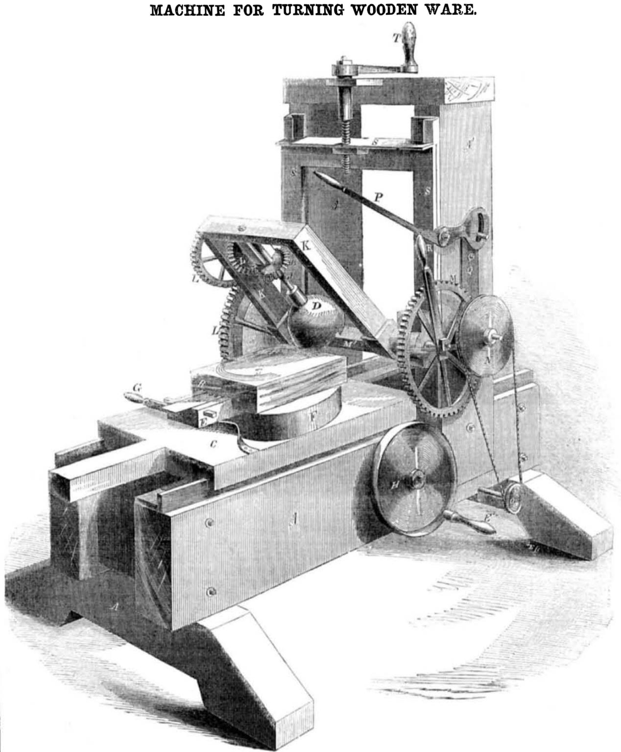
Only one cutter, D, is shown in fig. 1, but there are, in reality, several. They are of spherical shell-shape, placed one within the other, but all attached to the shaft, J.
