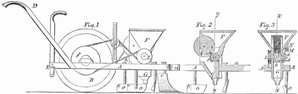
The concave, J, prevents the seeds falling in too scattering a manner as it drops through the spout, G, into the narrow furrow made by the drill, and is covered by the shares, O O said shares within the space cleared by the double share, C, and the wheel, B, passes over and presses the earth on the seed.
