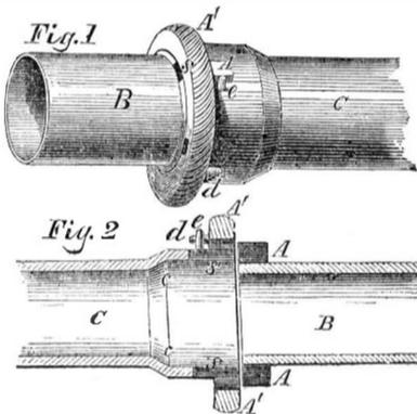
for when these pins are out of contact it is a sign that the sections of pipe are coupled, and vice versa. They are, therefore, coupling gauges, and in this character are very useful. This coupling can be made as strong as any in common use, and it can be more quickly operated than the common screw couplings.
