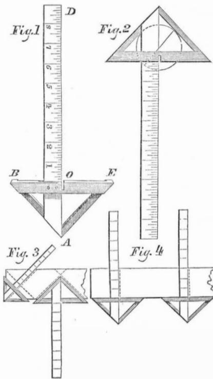
The application of the instrument as a graduated rule, T-square, and try-square, will be easily understood by inspecting fig. 4.
