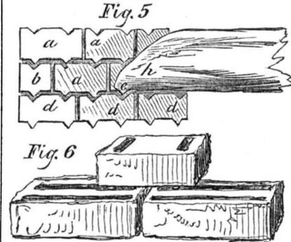
"It will be perceived at once that in bricks made upon this plan, the improvements will consist, 1st, in the greater security and strength of the walls locked and bound together by this device. 2nd, the bricklayer is enabled to lay several courses without the use of the line, and with much greater rapidity and accuracy than with common brick, it being scarcely possible to go wrong; and, 3rd, the spaces for mortar between the bricks are necessarily uniform, exact, and equal.
