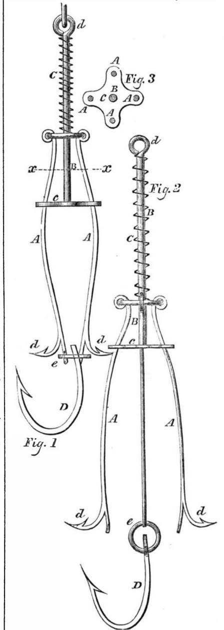
bring the barbs or hooks *d d*, between his jaws, and then pulls slightly upon the bait hook, D, it will be sprung, as shown in fig. 2, or unset, and the barbs, by the action of the spiral spring, C, caused to move laterally from each other, and consequently take into the top, bottom, and sides of the fish's mouth, and confine him securely, and thus relieve the bait hook of nearly all the strain.
