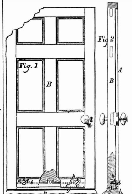
the bar, C, may be lowered by adjusting the set screws, d, which secure the bar in the groove, b, in the lower edge of the door. The heads of the set screws may be of any proper form so as to be rather ornamental than otherwise.
