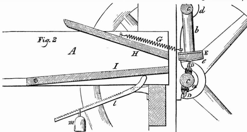
the front end of the feed box, A. The under surface of the bed, E, is provided with a layer of raw-hide, e, or other suitable material in order to prevent the edges of the knives from being injured by coming in contact with the bed. I is an adjustable throat piece, the inner end being secured to the sides of the feed box by pivots so as to allow the outer end to be raised or lowered to govern the length of the cut.
