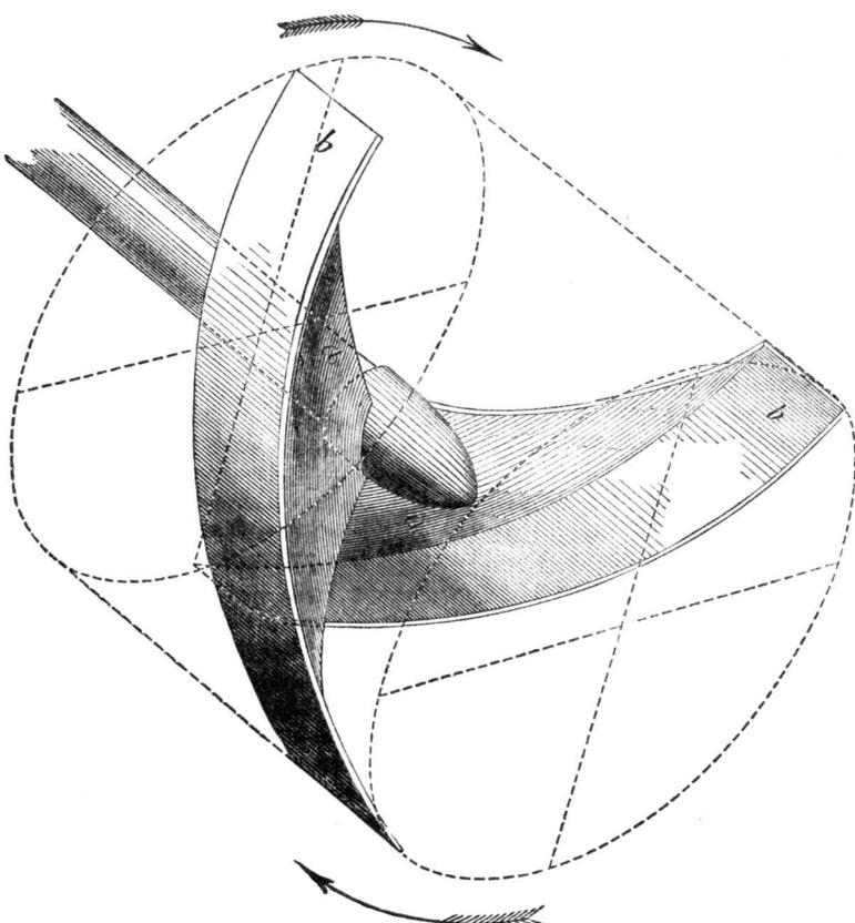
This figure is a perspective view of a new propeller for vessels, for which a patent was granted to Wm. F. Tyson, of Tamaqua, Pa., on June 21, 1853.
