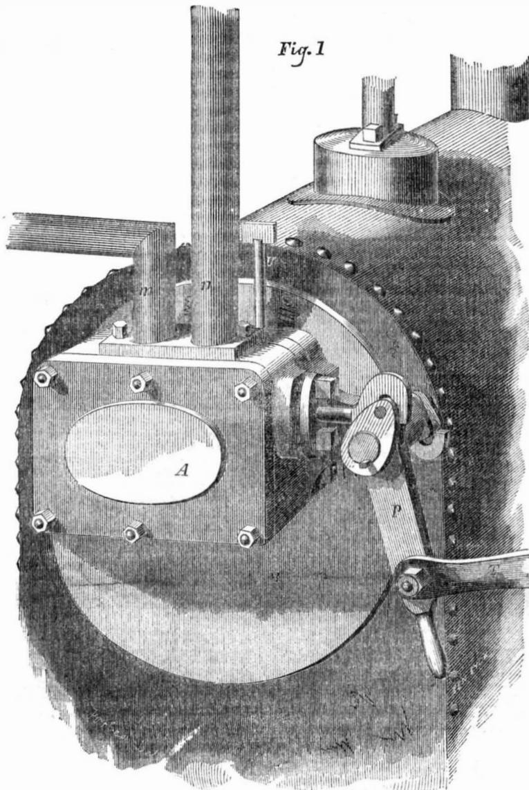
Figure 1 is a perspective view of an apparatus for supplying steam boilers with water, for which a patent was granted to Benjamin F. Bee, on the first of August last, to which he has given the title of Hydrestant. Figs. 2 and 3 are sectional views of the apparatus, showing the internal arrangements and the different positions the two valves are made to occupy, by which contrivance water is supplied to the boiler in proportion to the demand.
