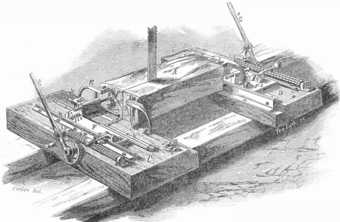
Motion is now given to the carriage, and the saw—a part of which is shown—is put in motion in the usual way when the slab on the outside of the log will be cut off, the log is then run back, and set by a transverse movement of the sliding dogs along the blocks, the detents, H H<sup>2</sup>, being previously lifted, and the fixed dog, D, withdrawn from the log. As soon as the transverse movement of the log begins, the detent is allowed to rest upon the notch rib of the gauge bar, and will drop
