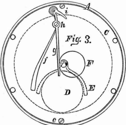
having a cylindrical weight placed within its case, said weight being detached, and from its gravity remaining stationary (not revolving with the wheel) and thereby giving motion to the working parts, as the wheel revolves.
