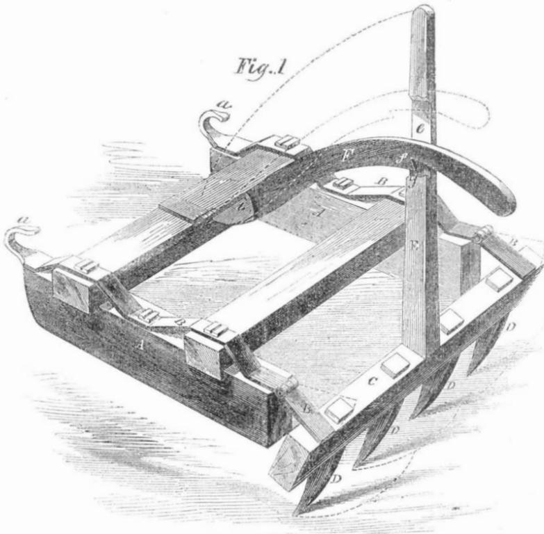
On the 29th of August last a patent was granted to Abraham R. Hurst, of Harrisburg, Pa., for the improvement in manure excavators represented by the annexed figure, which is a perspective view. The object of the implement is to loosen the manure to allow of its being easily shovelled.
