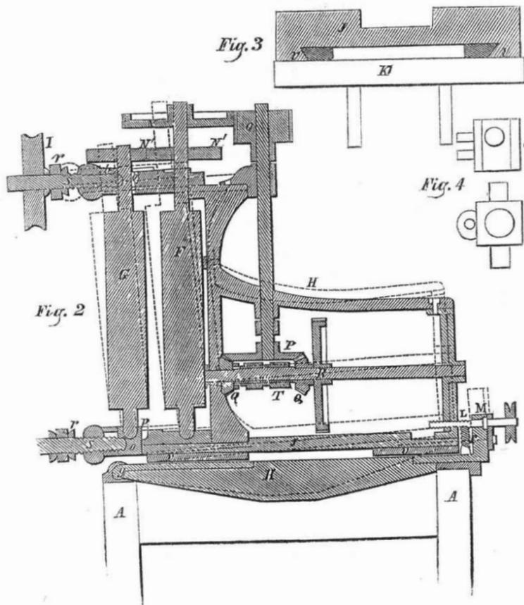
between guides upon a bed plate, K, attached transversely to the upper part of the frame, A, figure 3. The frame, H, may be moved when necessary by means of a screw, L, which passes through a lug or projection, M, at one
