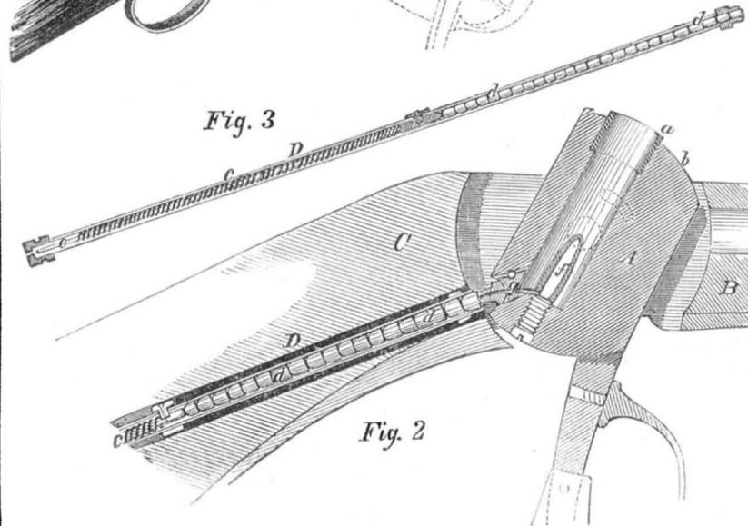
barrel, so as to prevent windage, and give the same advantage as the Minie ball does to muzzle loaders. It can also be charged with powder and patch, and no cartridge used, if desired, as this breech chamber is loaded like a common shot gun. We are assured by the Company, that this rifle possesses "one-third greater penetrating power, with one sixth less powder than any muzzle loading one.— A ball fired from this rifle has penetrated
