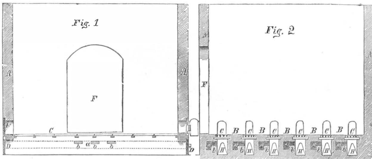
A patent was granted on the 4th of last July, to John S. Speights, of Baltimore, Md., for the improvement in Brick Kilns, represented in these engravings, fig. 1 being a longitudinal vertical section, and fig. 2 a transverse vertical section of the kiln. This is a coal-burning kiln, and the improvement consists in a certain arrangement of the fire grates, and air passages, whereby very perfect combustion of the fuel is obtained, and regulated at all parts of the kiln.
