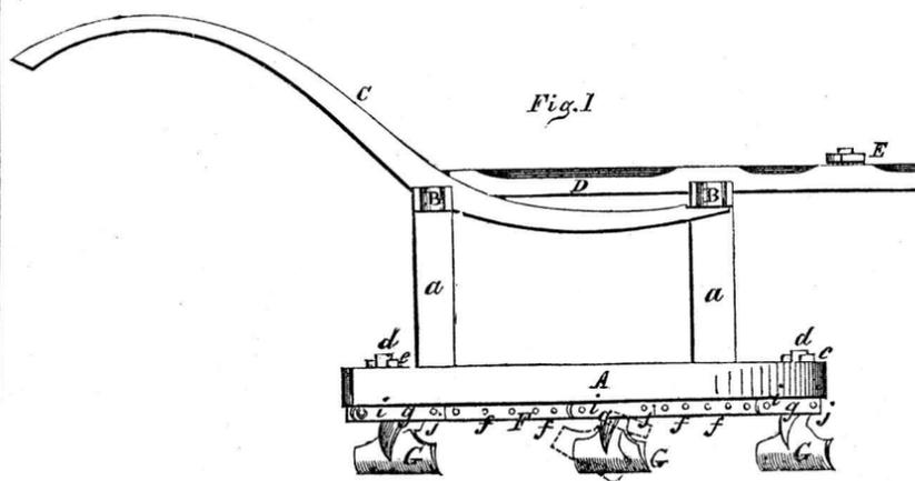
The annexed engraving is a side view of a Cultivator, for which a patent was granted to Griffith Lichtenthaler, of Limestoneville, Pa., on the 25th of July last. The nature of the improvement in this cultivator consists in the peculiar manner of attaching the shares to the beams, whereby they (the shares) may be readily adjusted in position, and also allowed to yield to any obstructions with which they may come in contact.
