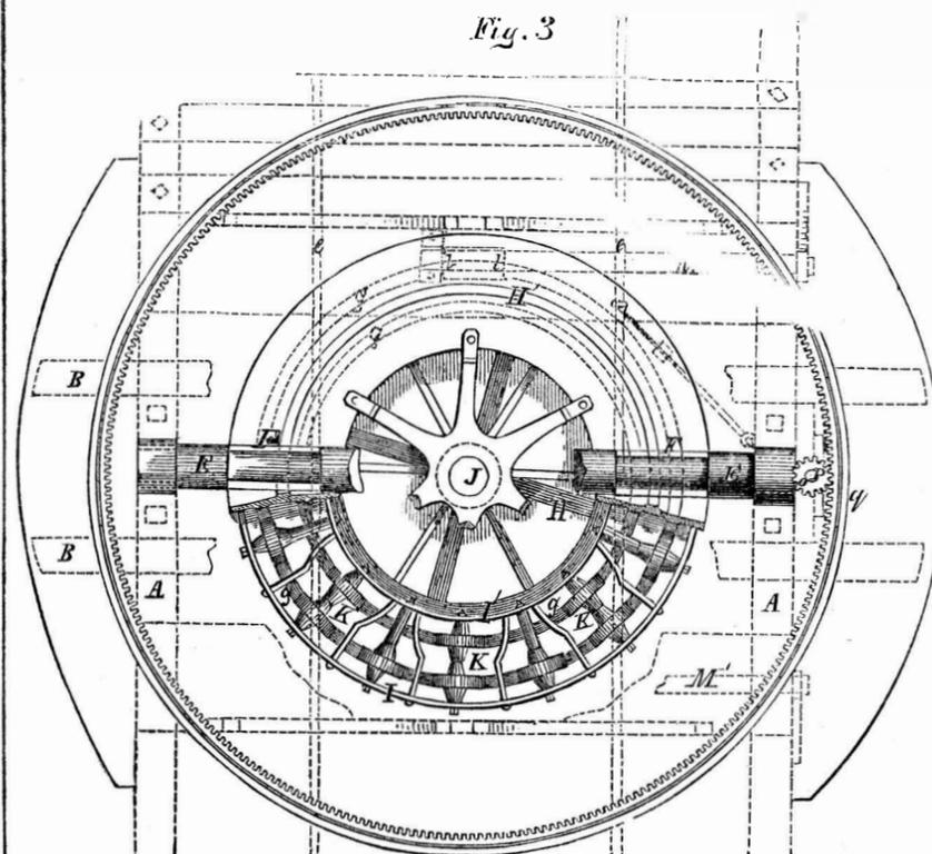
they are made eccentric to the journals. Upon the top side of the upper roller plate, *H'*, are two raised pieces which form bearings for the eccentric parts of *M M'* to rest upon.—Each of these shafts has a lever attached at its outer end, as shown in fig. 2, which can be
