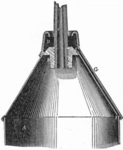
also frequently takes place at the side tube used for filling. The tin tube being soldered to the cap, when any sediment from the oil gets into the tube and stops its running, it has to be forced back into the can by means of a wire, and of course is liable to trouble again. The tin tubed cans and all others however constructed, except this, are frequently covered with oil, dripping down on the outside, rendering them dirty, and wasting much oil.
