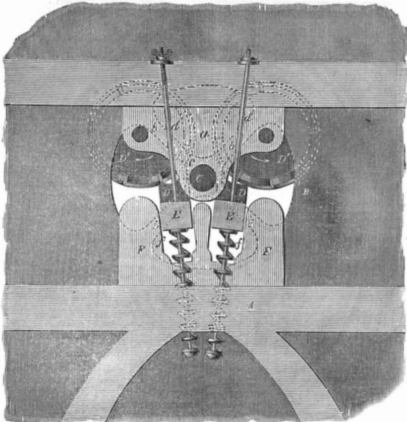
The annexed engraving is a vertical transverse section of an improvement in machinery for cutting or grinding woolen rags, &c., into fine flocks. The inventor is Joseph N. Pitts, of Blackstone, Mass., who has taken measures to secure a patent. The nature of the improvement consists in combining and arranging within a revolving cylinder two inward revolving rollers which have spiral cutters on their peripheries. These act in combination with one another, and with two stationary adjustable cut-
