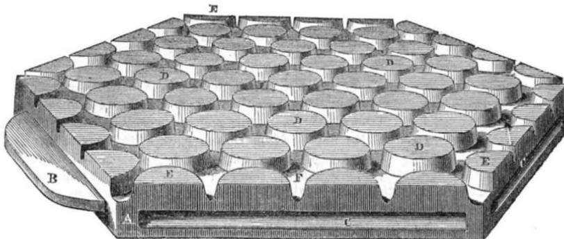
To supersede the ordinary Russ paving for streets, a new arrangement by means of cast-iron blocks has been invented by L. Colwell, of New York City, who has taken measures to secure a patent. The above engraving is a perspective view of one of the blocks forming a section of the paving and displays the structure and arrangement of this new method. Each of these blocks is six-sided, being in shape a regular hexagon, so that they are easily fitted one to another.
