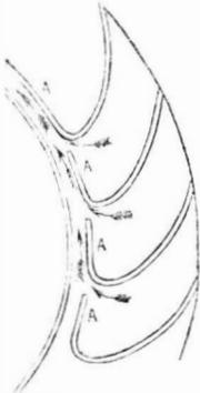
**BREAST WHEEL WITH CLOSE SOLE AND VENTILATED BUCKETS.**—This wheel is adapted for heights not exceeding 18 or 20 feet, and where it is subjected to back water. Every wheel of this kind should have capacity in the buckets to receive a sufficient quantity of water to force the wheel at full speed through a depth of five or six feet of backwater.
