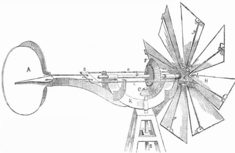
This improvement in Wind-mills relates to a superior mode of governing the vanes according to the velocity of the wind. It is the invention of Mr. Marvin Smith, of New Haven, Conn., who has taken measures to secure a patent for the same. Figure 1 is a perspective view, and figure 2 is a plan view:—the same letters refer to like parts.
