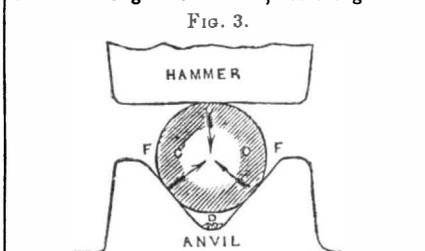
surface of junction it occupies. The frequency of this interposing scoria as the true cause of unsound forged work, was forcibly alluded to by Mr. Nasmyth, and shown to be the most fertile source and cause of the failure of wrought iron work, resulting as such too frequently does in the most sad and disastrous accidents—such as the failure of the links of chains and anchors, and in the costly and often distressing results arising from defective (i. e. blistered) boiler-plates.
