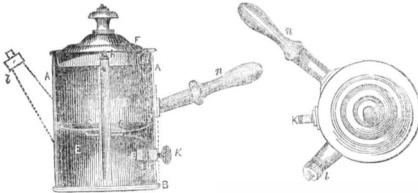
This apparatus is made upon what is called the water-spout principle. Water is boiled in the lower part of the vessel and by the expulsion of the air from the upper part by the steam, a column of boiling water rises through a tube in the centre of the vessel and is thrown over the coffee in the upper vessel by a dash plate. The coffee is placed upon a perforated plate, or false bottom, and its pure, not its astringent part, is thus better extracted than by boiling, or simply scalding.
