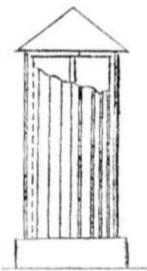
This is another arrangement of the Air Mill a cut of which appeared in No. 4, of this volume. The arrangement here is to show that by protecting one half of the sails supported on a perpendicular shaft by means of a circular casement of shutters, a similar effect is produced to that represented in No. 4. It is our opinion, however, that neither this nor the other modification of a windmill, are as efficient as the old and simple plan.
