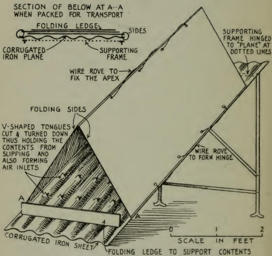
PORTABLE INCLINED-PLANE INCINERATOR
