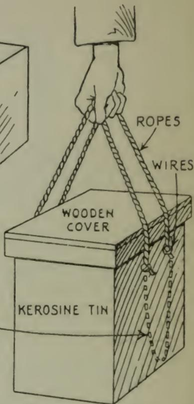
METHOD OF REMOVING TIN FOR EMPTYING
