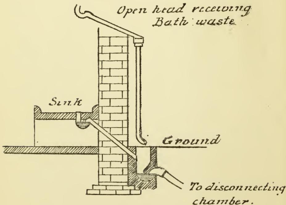
FIG. 4.—A KITCHEN SINK, PROPERLY DISCONNECTED
