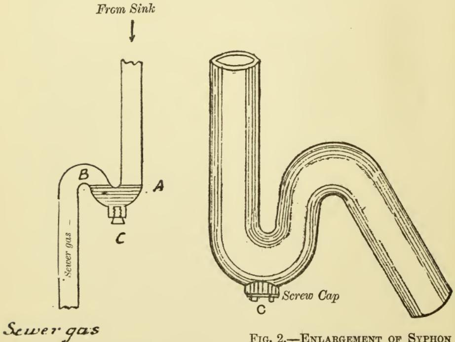
FIG. 1.—LEAD SYPHON (OR S) TRAP, WITH SCREW CAP FOR CLEANSING (Corfield).
