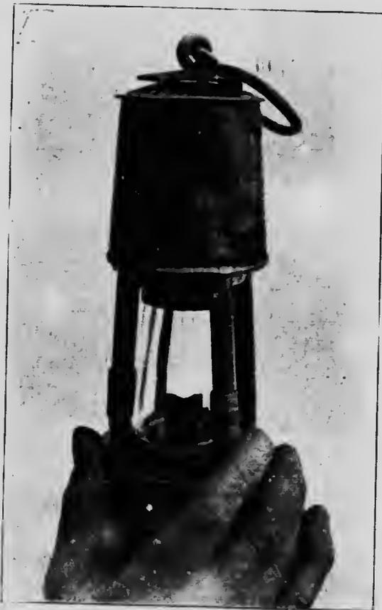
FIG. VIII.—Ashworth's patent Gray, Deputy or Fireman's Lamp. Showing mode of manipulation when testing for firedamp.
