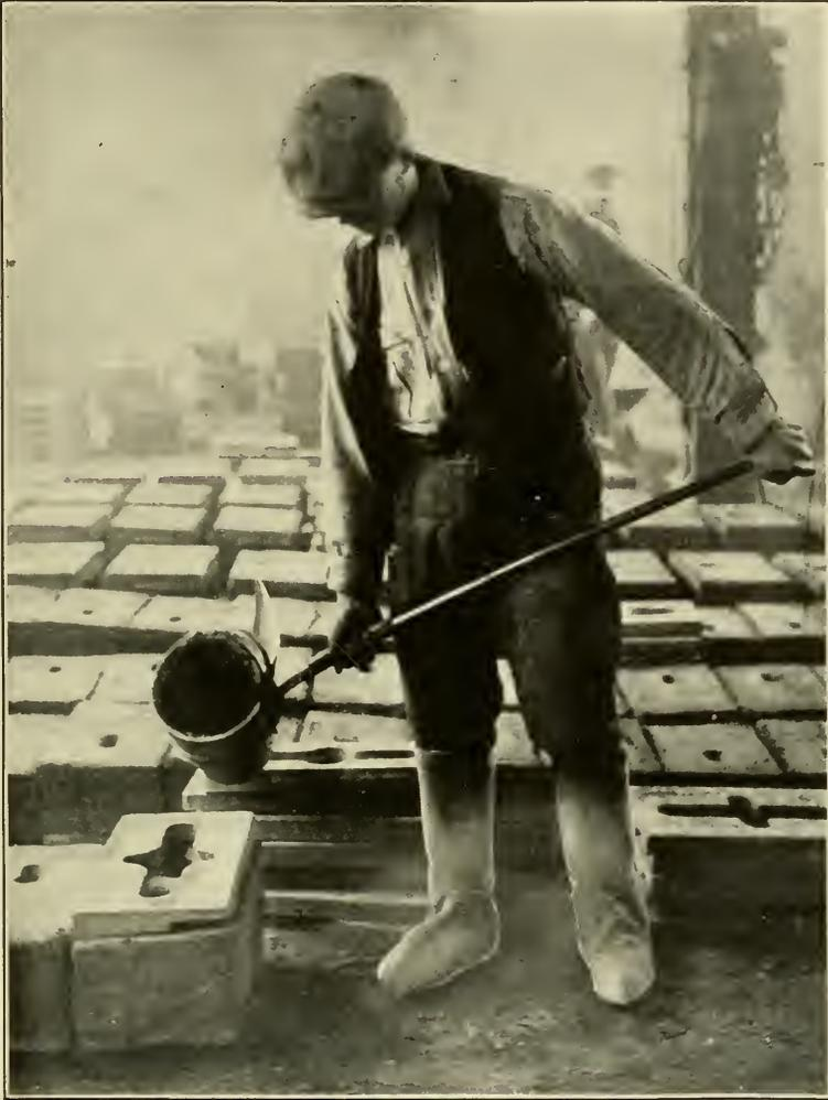
FIG. 4. POURING FROM A HAND LADLE.
