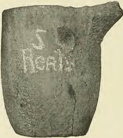
FIG. 8. THE CRACK IN THIS CRUCIBLE DEVELOPED AFTER FIVE HEATS.
