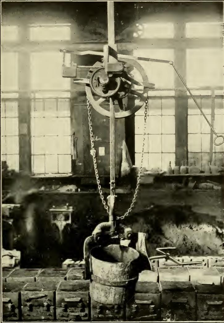
FIG. 6. A CONVENIENT LABOR-SAVING POURING DEVICE.
