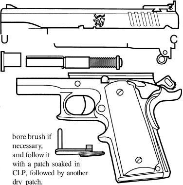
With a quality lubricant designed for stainless steel (such as FP-10, Energy Release, etc.), put a few drops on the running, or function, surfaces *in the slide only;* i.e., where the barrel rides, the slide rail surfaces where they match the frame, and on the disconnector ramp. These areas usually show wear and shiny patches. NEVER squirt oil into the frame.
