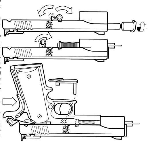
**NOTE:** Do not try to align the barrel link, the disassembly notch and the top of the slide stop all at the same time. Align the link first, insert the slide stop shaft, and then rotate the slide stop upward until it aligns with the disassembly notch.
