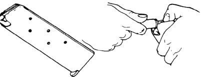
of a cartridge down against the front end of the follower and slide backward in one smooth motion under the retaining lips.
