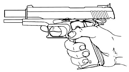
This feature tells the shooter that his pistol is empty, and permits rapid reloading. Press the slide stop down out of its locking notch to allow the slide to move forward. If a loaded magazine is inserted and the slide stop is pushed down, the slide will load a fresh cartridge from the magazine into the chamber, and the pistol is ready to fire.
