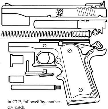
With a quality lubricant designed for stainless steel (such as FP-10, Energy Release, etc.) put a few drops on the running, or friction, surfaces *in the slide only;* i.e., where the barrel rides, the slide rail surfaces where they match the frame, and on the disconnector ramp. These areas usually show wear and shiny patches. NEVER squirt oil into the frame.
