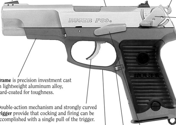
When ambidextrous **manual safety** is in "safe" position, the firing pin is cammed forward into the slide. This simultaneously places the firing pin out of reach of the hammer and locks the firing pin in a neutral position, preventing the firing pin from movement toward the cartridge. Further, the entire firing mechanism is completely disengaged from trigger.
