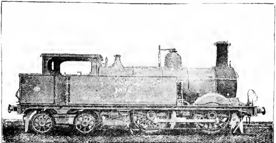
FOUR-WHEELED COUPLED BOGIE PASSENGER TANK ENGINE.
