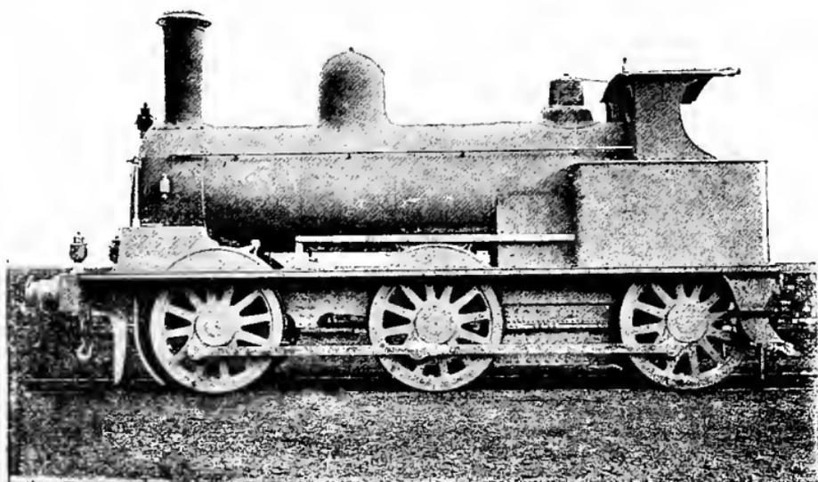
COAL ENGINE. SIX COUPLED WHEELS FOUR FEET THREE INCHES.
