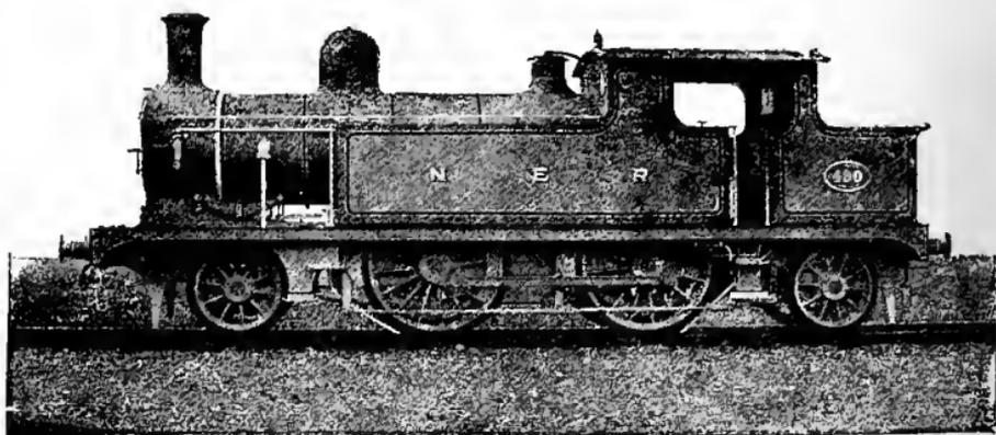
Passenger side tank engine, designed by Mr. T. W. Worsdell, 4-coupled 5 feet 6 inch wheels, 18-inch cylinders, and 24 inch stroke, built in 1886 for local passenger trains; it has 4 intermediate wheels coupled, and a pair of wheels with radial axle-box at each end.
