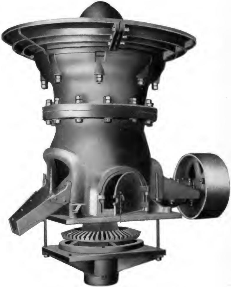
McCully Gyratory Crusher—Standard Discharge.
