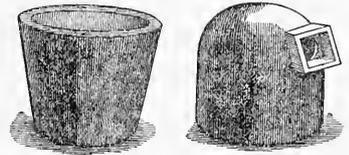
SHAPE OF POTS.—Pots for all glass but flint are open truncated cones, the smallest diameter being at the bottom. Even some flint-glass pots are used uncovered in the gas furnaces, but usually they are covered as represented in the accompanying cuts.
