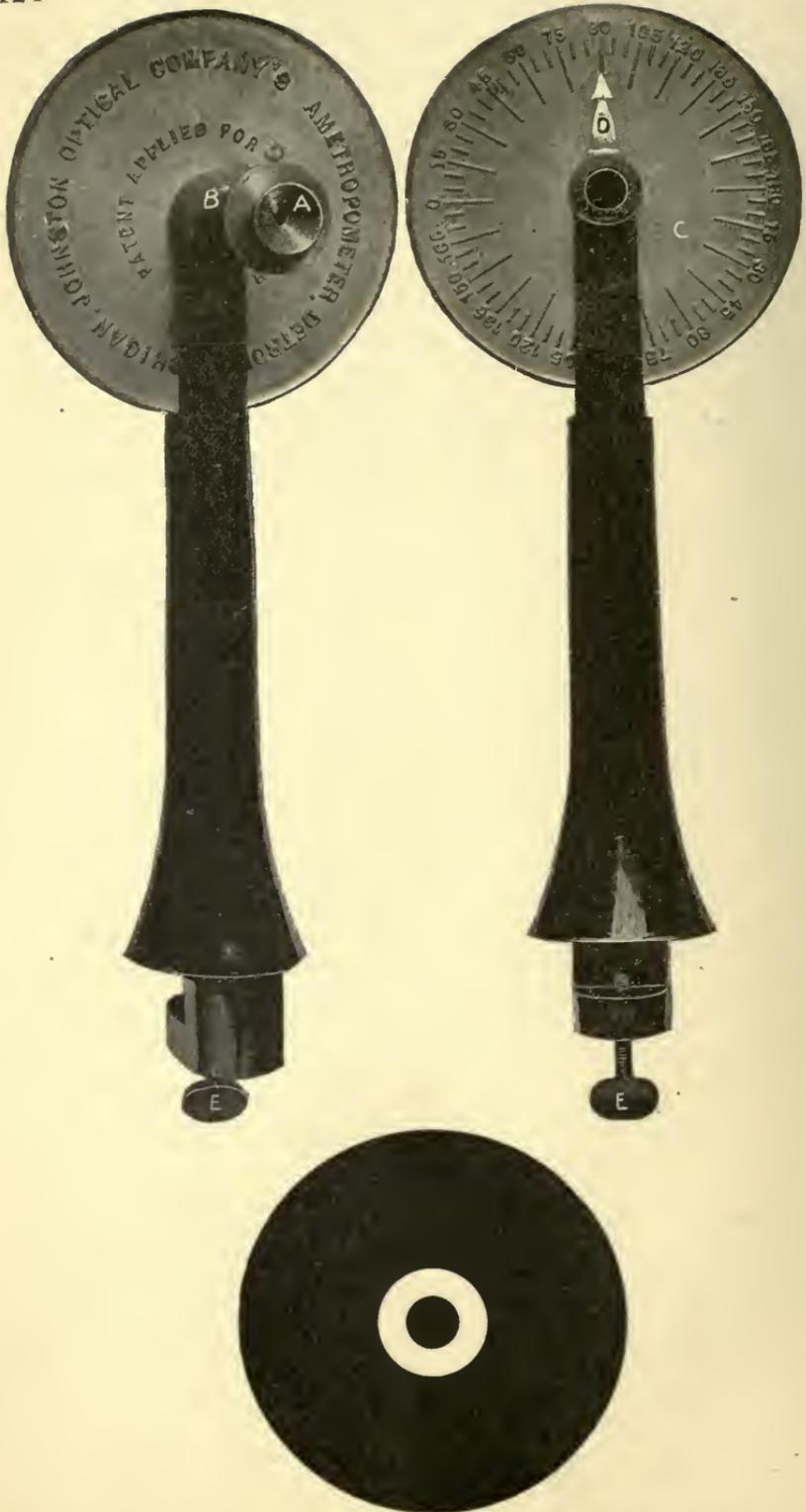
FIG. 72.—Showing Ametropometer.
