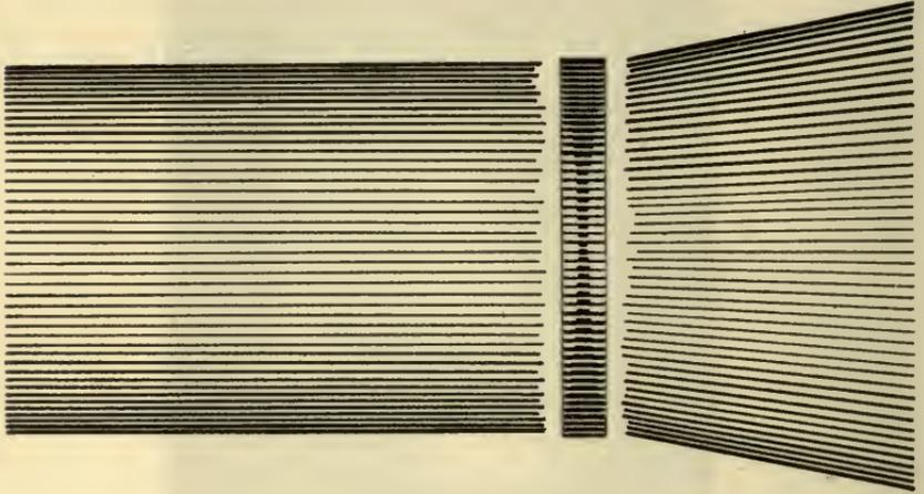
FIG. 7.—Showing the Divergence of a Beam of Light in Passing Through a Spherical Bi-Concave Lens.
