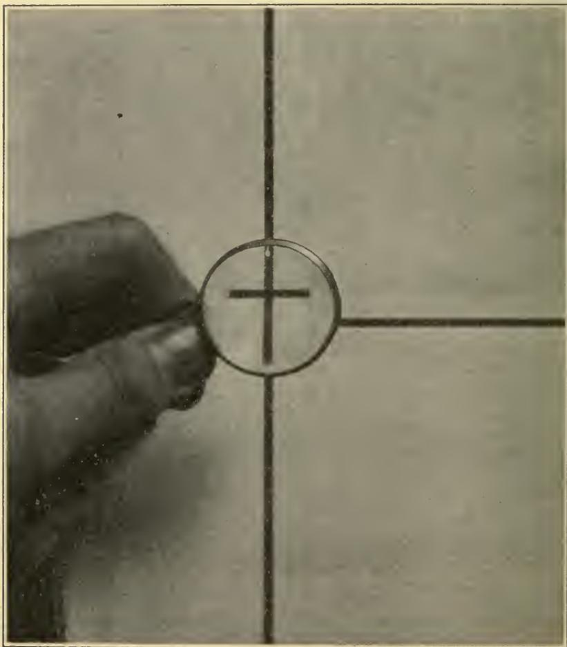
FIG. 19.—Showing the Effect of a Prismatic Lens.
