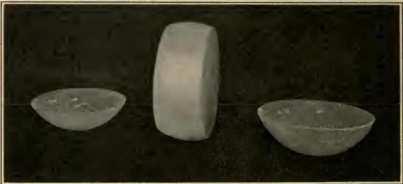
FIG. 4.—Showing Sections of a Sphere to Represent Convex Spherical Lenses.
