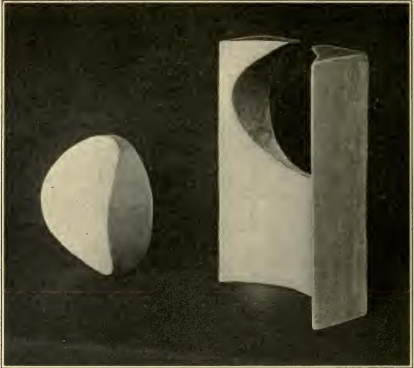
FIG. 15.—Showing a Concave Cylindric Lens.
