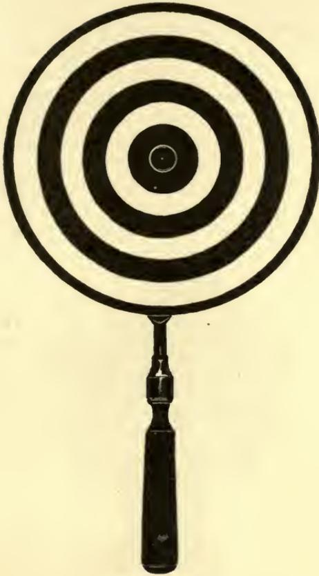
FIG. 74.—Showing Placido's Disc.
