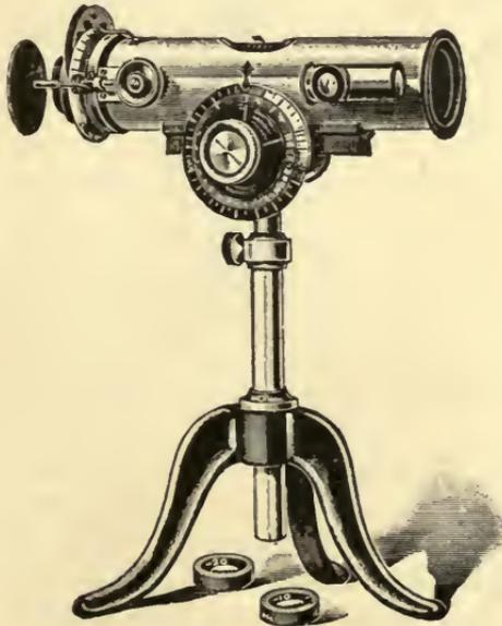
FIG. 73.—Showing Refractometer.
