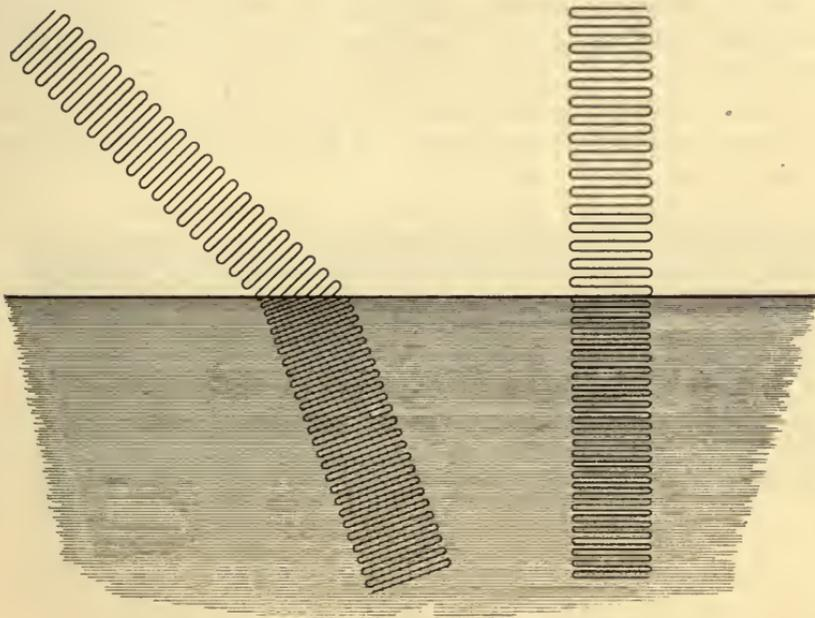
FIG. 1.—Showing the Refraction of a Light Wave.
