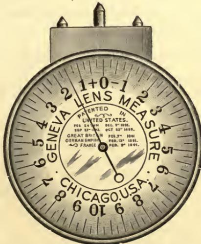
FIG. 21.—Showing a Lens Measure.
