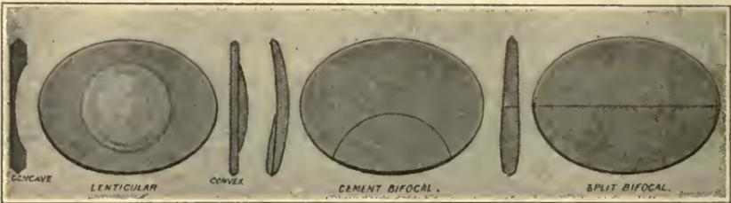
FIG. 65.—Showing Different Forms of Bifocal Lenses.
