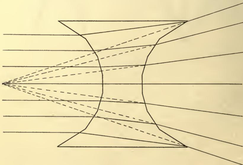
FIG. 11.—Showing Concave Spherical Surfaces as made up of Prism Sides.
