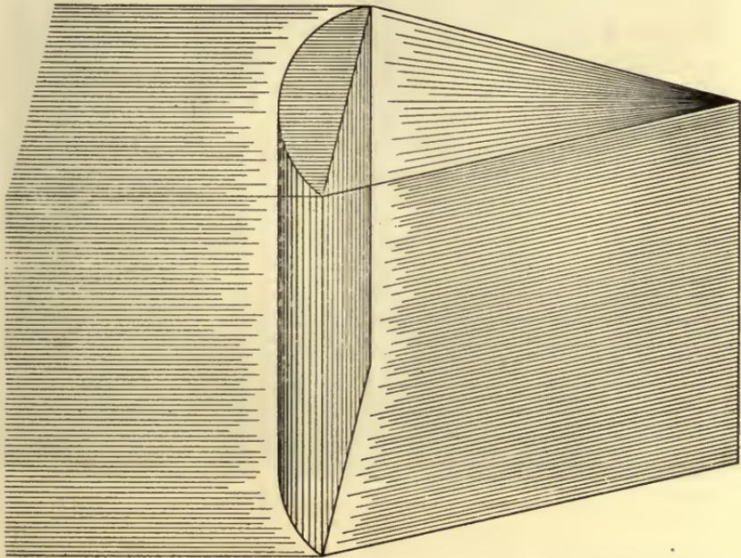
FIG. 14.—Showing Effect on a Beam of Light Passing Through a Cylindric Lens.
