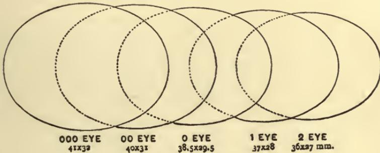
FIG. 60.—Showing Standard Lens Sizes.
