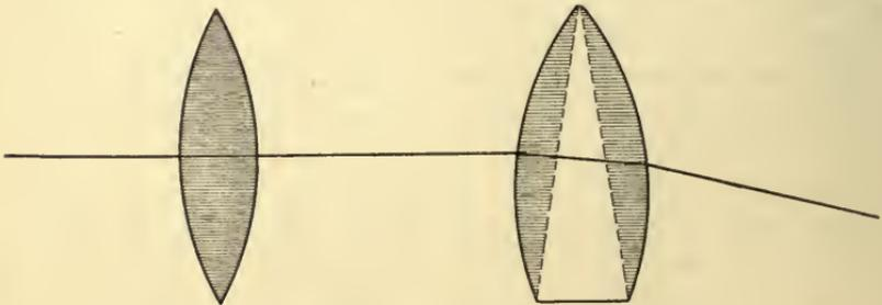
FIG. 22.—Showing Prismatic Effect of Decentering a Lens.
