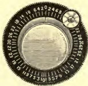
FIG. 76.—Showing Risley's Rotating Prism.
