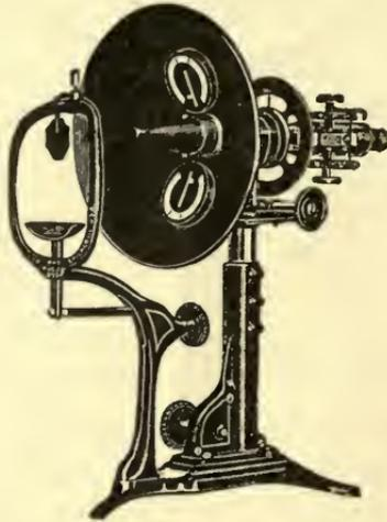
FIG. 75.—Showing Type of Improved Ophthalmometer.
