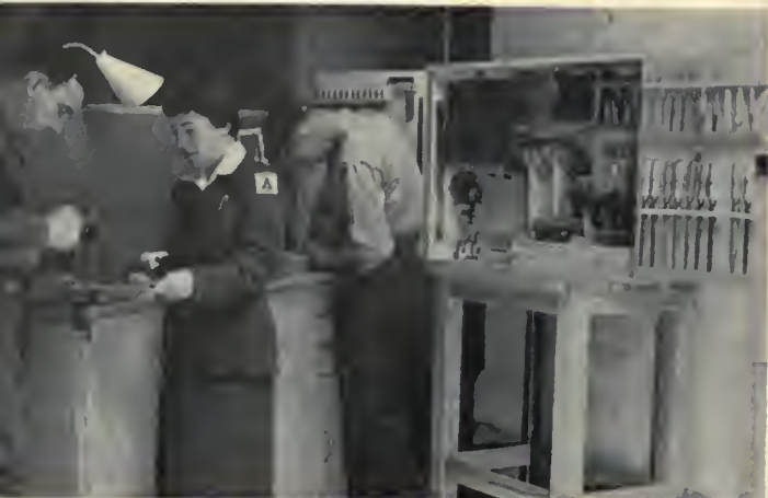
A movable crafts bar, designed for limited quarters, has storage space for supplies and hand tools and a small work area.
